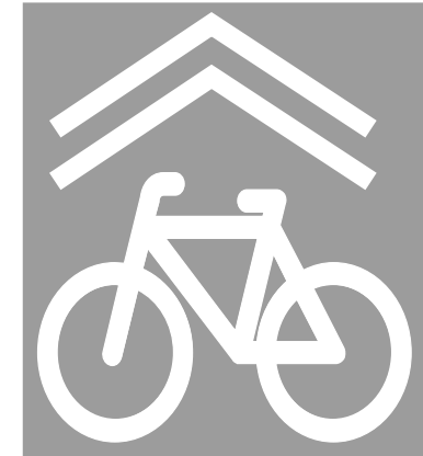
Shared lane pavement marking or “sharrow”
