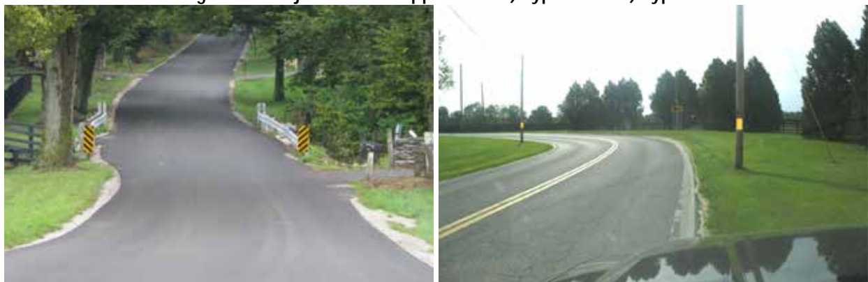
Figure 16: Object Marker Application a) Type 3 and b) Type 2
