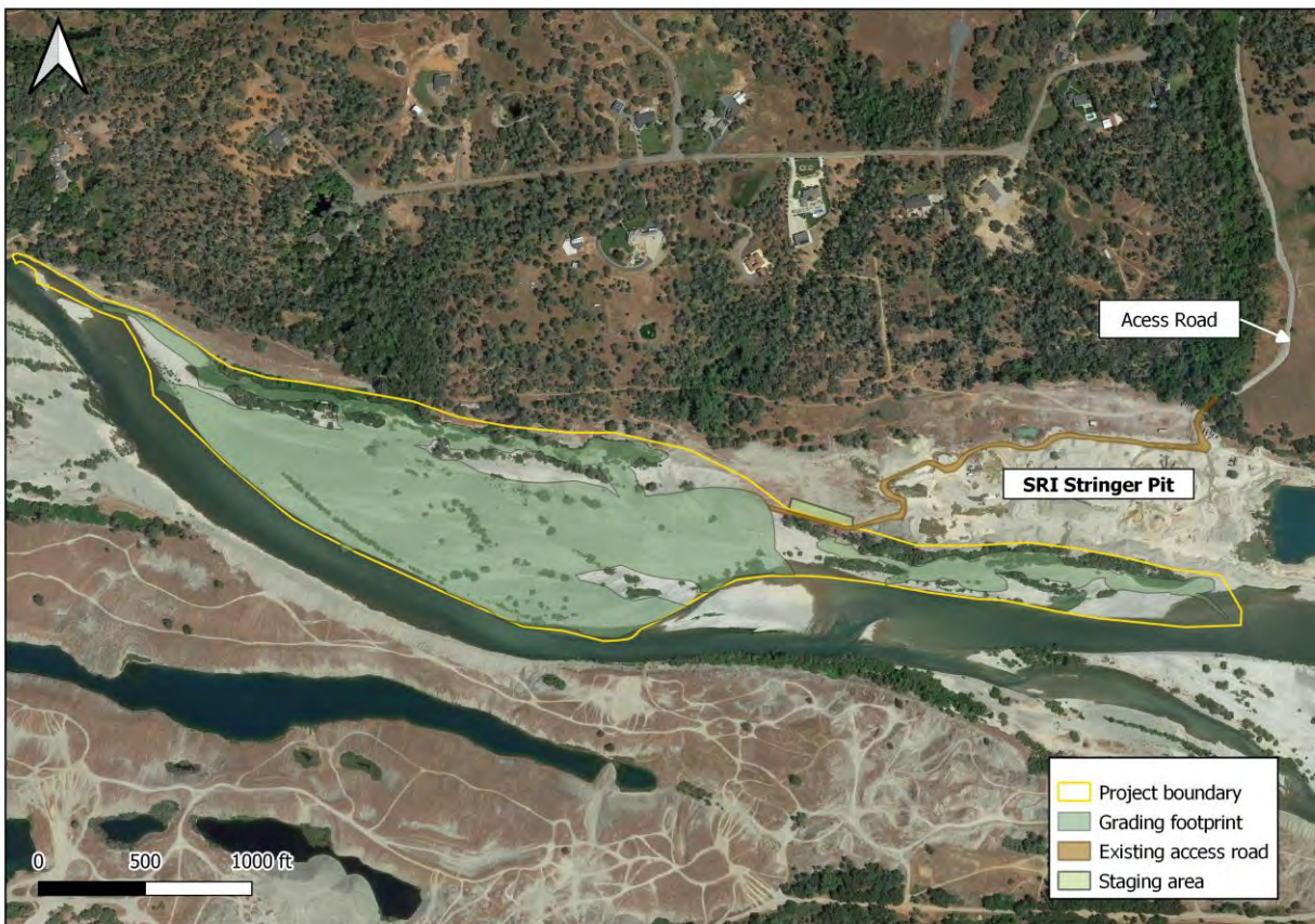
Figure 3. The existing access road and staging area to be used for construction of the Proposed Action.
