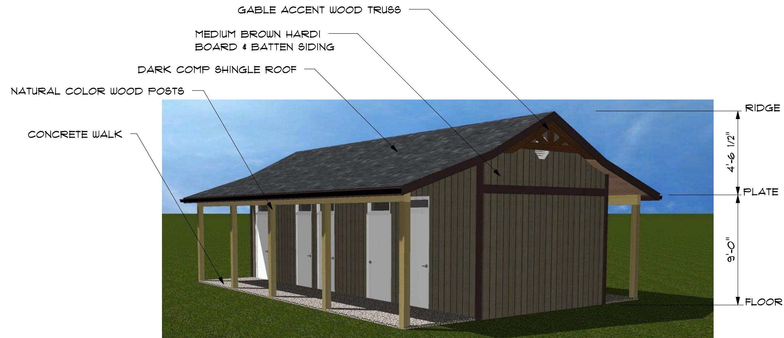
FRONT RIGHT ELEVATION (NORTH/WEST)
