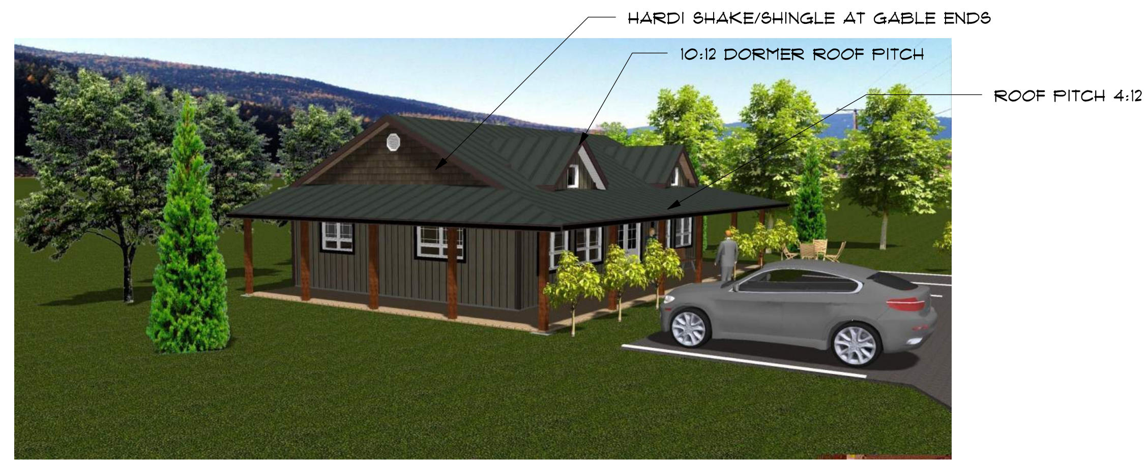
FRONT LEFT ELEVATION (NORTH/EAST)
