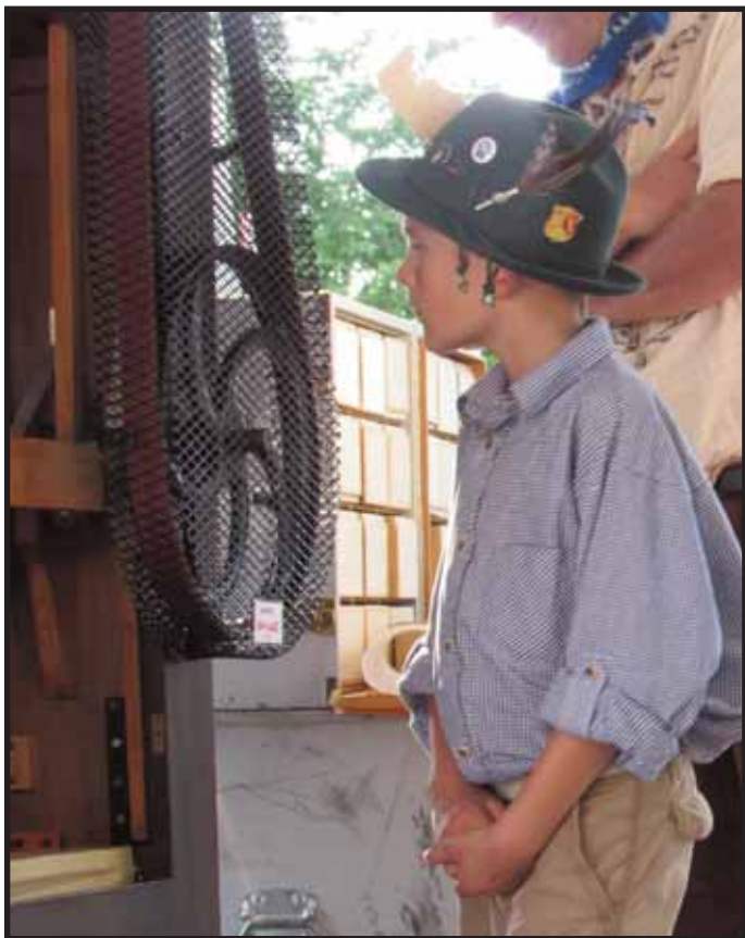
Figure 52. A youngster’s mischievous fingers can’t reach the flat drive pulley thanks to the newly-installed belt guard.
