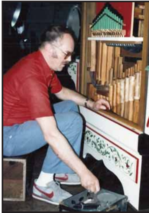
Figure 40. Lance Johnson regulates the trumpet pipes that are shaded by the organ case skid.
