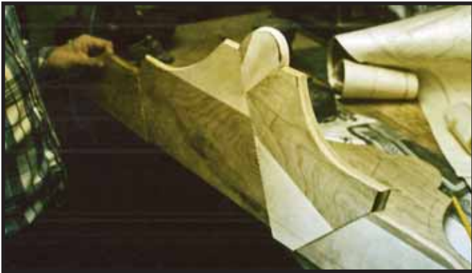
Figure 36. The crown design using Ruth curves was routed in pieces to allow for inside corners, then assembled.
