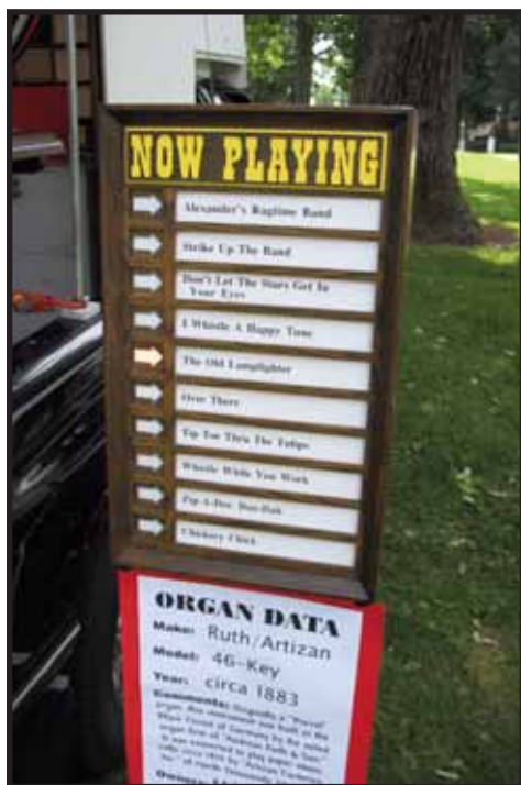
Figure 47. The automatic “Now Playing” display sign with interchangeable title cards. The organ roll’s coin trip perforation advances the lighted arrow.
