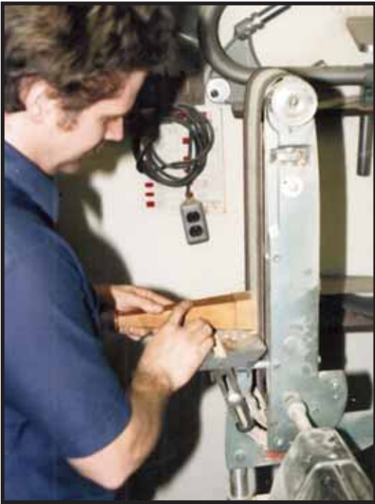
Figure 39. Mike sands smooth an extended trumpet resonator after pipe voicer, Lance Johnson, instructed him to remove half an inch of length.
