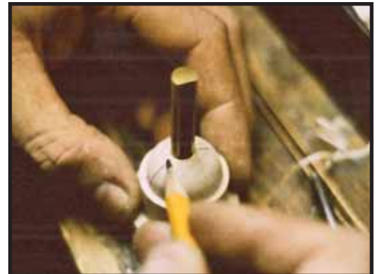
Figure 29. Foot block for the new trumpet pipe replicates the Ruth original.
