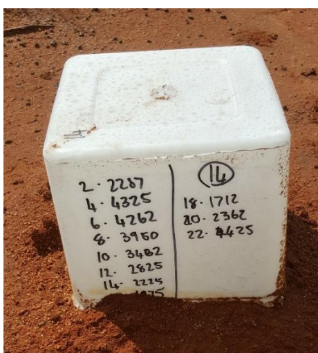
Figure 43: Plastic container covering applied beetles and dung. Ventilated at the sides with mesh (not visible in picture). Numbering on the front facing side of the container indicate penetration resistance measurements in kPa.
