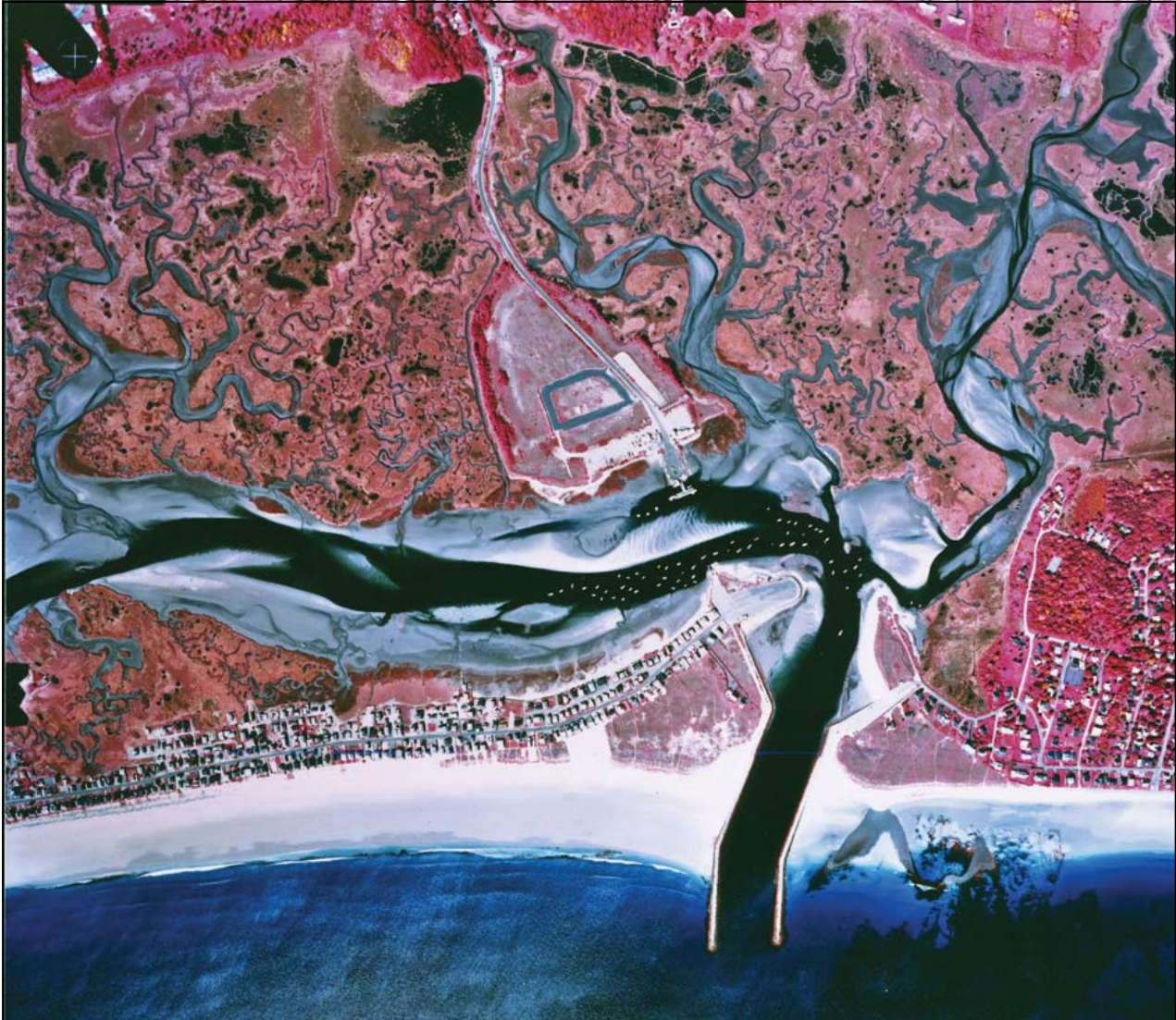
Aerial color-infrared photograph of the Webhannet River inlet showing beach, beach development, jetties, Wells harbor, filled marsh, natural marsh, and estuarine channels. Photo Wells NERR.
