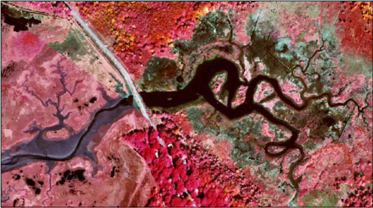
Aerial photo of impounded water behind Drakes Island Road, in the northern Webhannet Estuary, due to tidal restriction at the road. A self-regulating tide gate has since been installed. Photo Wells NERR.
