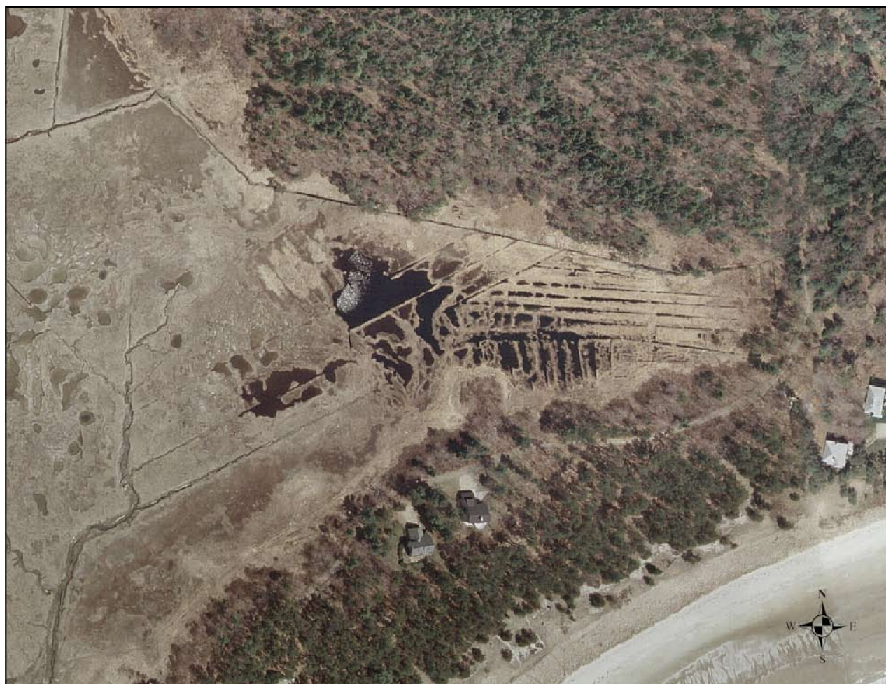
Example of marsh subsidence, in this case likely due to peat oxidation after extensive ditching reduced the original water table. After subsidence, water levels are higher than the marsh surface. Source Maine Office of GIS, 2003.
