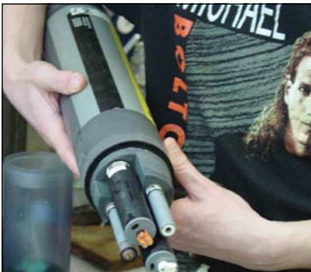
Close up of a YSI 6600-series water quality monitoring sonde used in the System Wide Monitoring Program. Photo Jeremy Miller.
