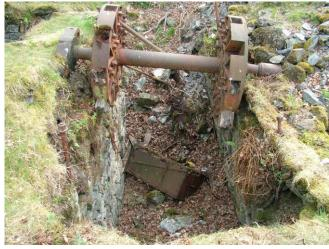
Slide 75 The axle of the 20 foot wheel, note tram wagon body in the bottom of the pit.
