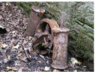
Slide 88 Flat rod wheel and rollers in the bottom of the wheelpit
