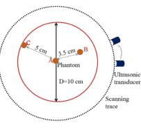
FIG. 7. (a) Experimental setup. DAQ, data acquisition circuits. (b) Top view of the scanning configuration.
