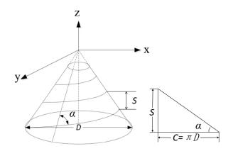
FIG. 1. The schematic of the conical logarithmic spiral structure.
