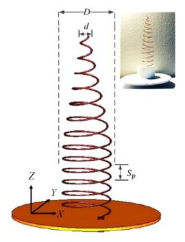
FIG. 3. The quasi-conical spiral structure (left) and the photograph of the antenna (right).
