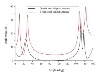
FIG. 4. The axial ratio of the antenna.
