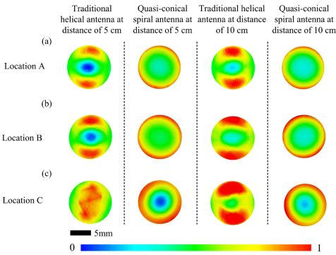
FIG. 6. The SAR distribution of the phantom at (a) location A, (b) location B, and (c) location C indicated in Fig. 7(b). The first and second rows show the SAR distribution images at the distance of 5 cm by the traditional helical antenna. The third and fourth rows show the SAR distribution images at the distance of 10 cm.
