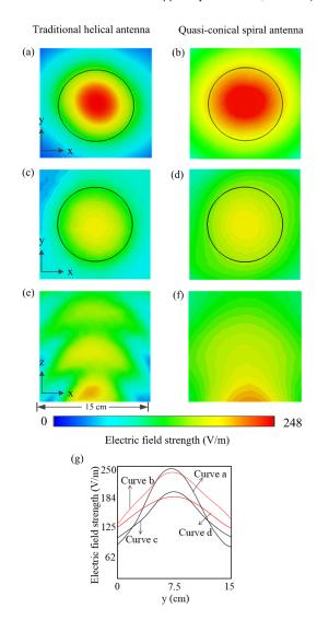
FIG. 5. Simulated distribution of the electric field produced by the traditional helical antenna [(a), (c), and (e)] and the quasi-conical spiral antenna [(b), (d), and (f)]. (a) and (b) The x-y cross section images at the distance of 5 cm. (c) and (d) The x-y cross section images at the distance of 10 cm. (e) and (f) The images along the z-axis from the distance 0 cm to 10 cm. (g) The electric field distribution along the line of x = 7.5 cm.
