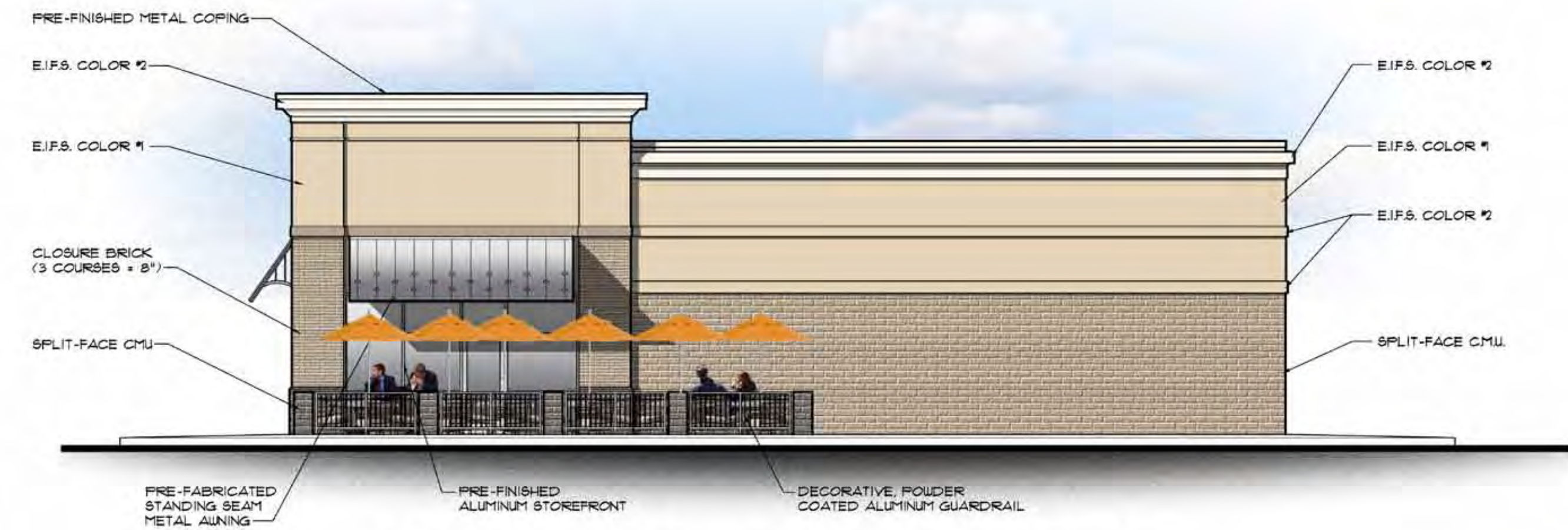
(B) RIGHT SIDE ELEVATION AREA A SCALE: 1/8" = 1'-0"
