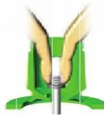
Figure 17 - Press In Seal
