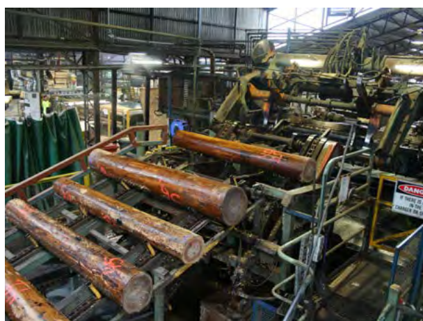
Eucalyptus cloeziana veneer billets ready for rotary peeling (Photo: R. McGavin)
