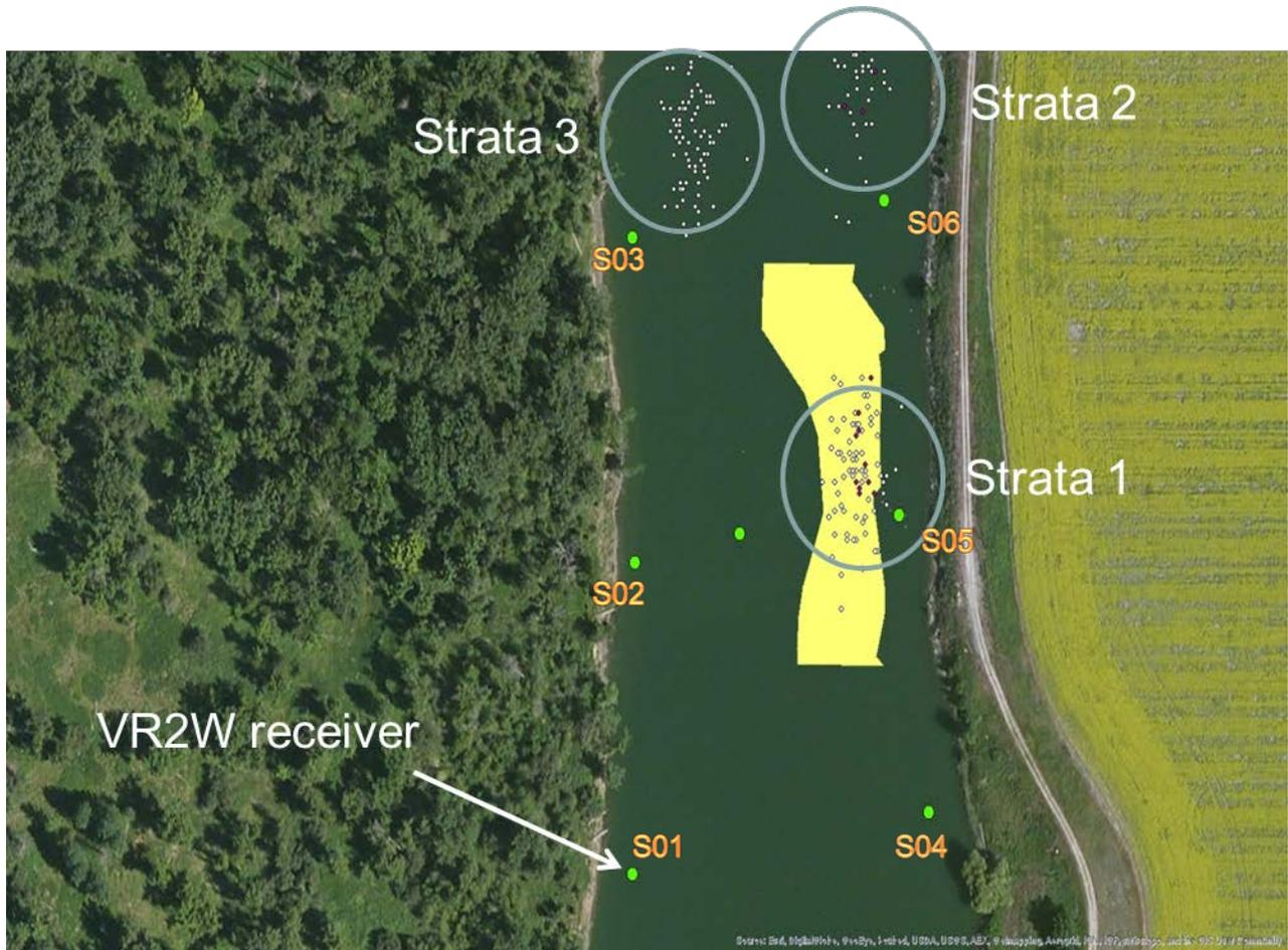
Figure 1.6. Substrate mat sampling design with reference to SEPP area at Shorty's Island. White dots within strata circles denote locations of substrate mats without eggs. Dark red dots within strata circles denote substrate mats containing eggs. Green dots on periphery denote location of Vemco VR2W receivers with co-located sync tags (orange labels) for VPS study.
