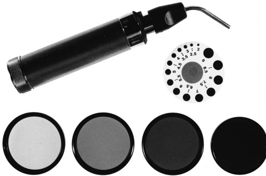
Figure 15.9. The equipment needed to quantify or bring out a relative afferent pupillary defect includes a bright handheld light source, a pupil gauge, and a set of photographic neutral density filters in 0.3, 0.6, 0.9, and 1.2 steps.
