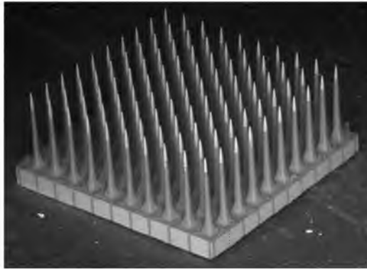
Fig 5.1 Scanning electron micrograph of the UEA with 100 (10 by 10) silicon electrodes.
