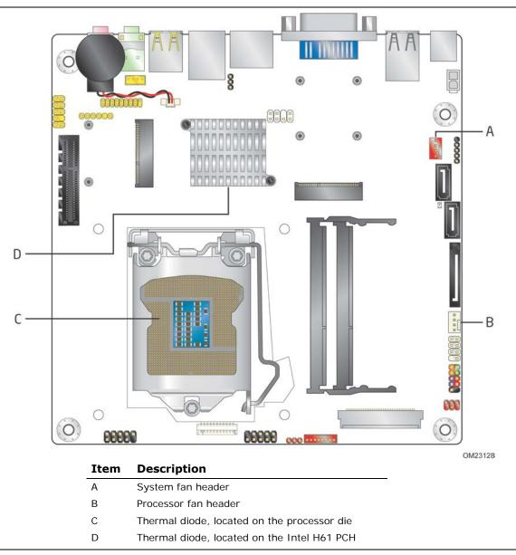
Figure 9. Thermal Sensors and Fan Headers
