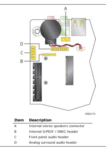
Figure 5 shows the location of the internal audio headers.
