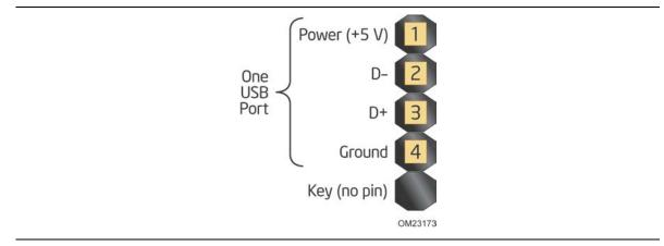
Figure 17. Connection Diagram for the Front Panel USB 2.0 Single-Port Header
