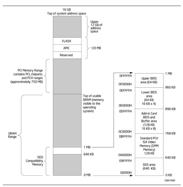
Figure 11. Detailed System Memory Address Map
