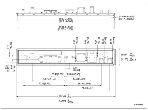
Figure 18. Half-Height Back Panel I/O Shield
