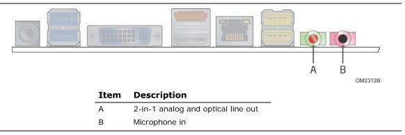
Figure 6. Back Panel Audio Connectors
