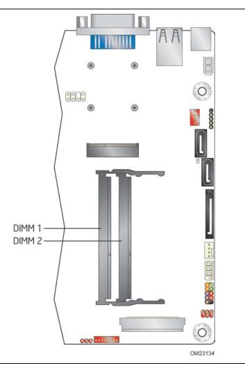
Figure 4 illustrates the memory channel and SO-DIMM configuration.
