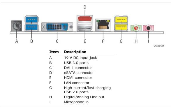
Figure 12. Back Panel Connectors
