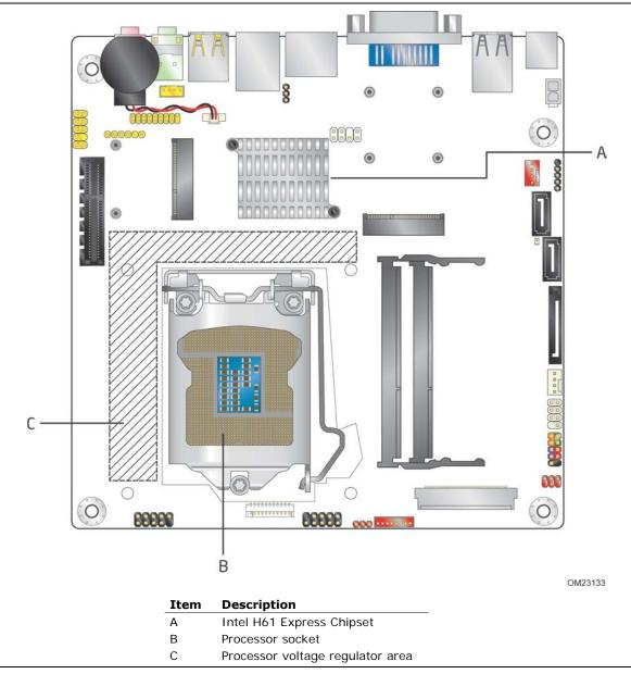
Figure 23. Localized High Temperature Zones
