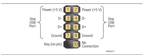
Figure 16. Connection Diagram for Front Panel USB 2.0 Dual-Port Headers
