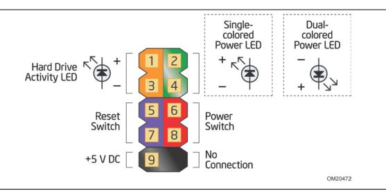
Figure 15. Connection Diagram for Front Panel Header
