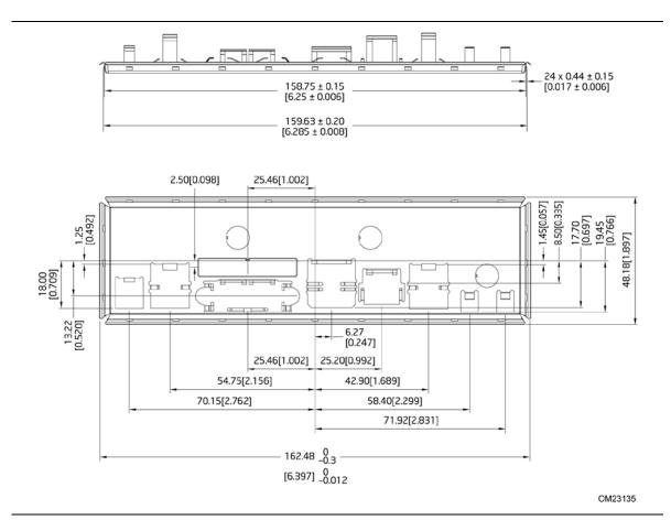
Figure 19. Standard-Height Back Panel I/O Shield
