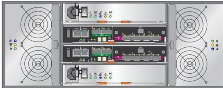
Figure 5) E5560 rear view showing dual controllers, power supplies, and cooling fans. In the DE6600 disk shelf, the controllers are replaced with Environmental Service Modules providing SAS connectivity.
