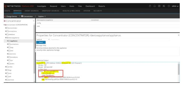
3. SSH to the Concentrator appliance or use iDRAC to connect to the console. Use **perccli** to create the virtual drive with installed Meta Pack kit. Create the Virtual Drive or Drive Group (DG) on the internal controller using the disks in slot 4 through 6 using the below command.
