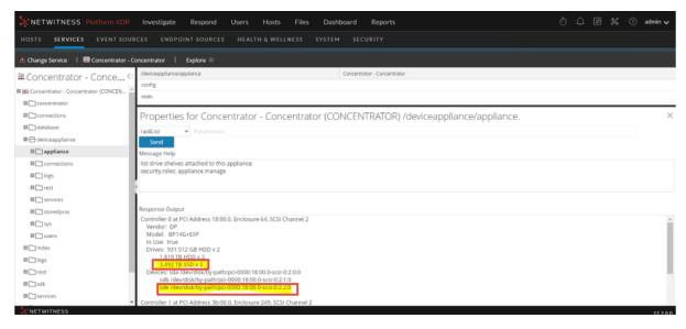
5. Execute the **partNew** command with the below parameters to create the new index partition on the block device (sde) created in earlier step:
