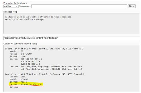
2. Execute the raidNew command with the following parameters using the controller number and the enclosure number you just recorded.
