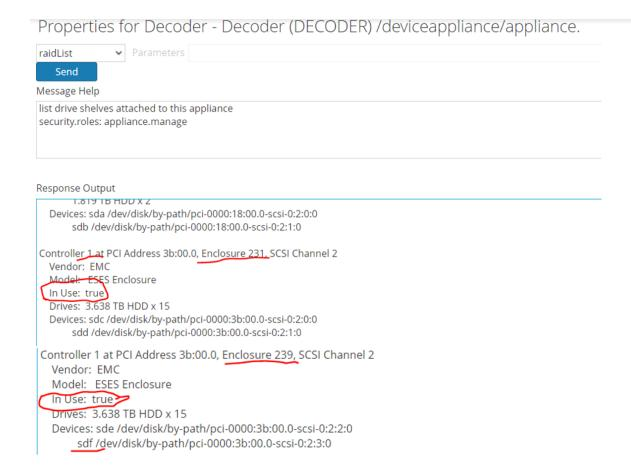
4. Use devlist to view the new block devices and their sizes. The new devices are highlighted in red.
