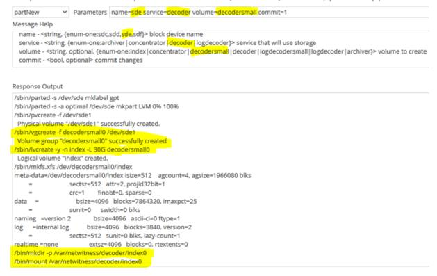
9. Execute the partNew command to create the packetdb decoder volume (Second Enclosure SDE, SDF) with the following parameters.
