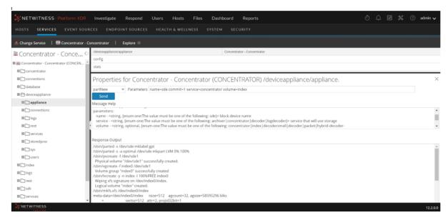
6. The concentrator appliance is already configured with a Power Vault (an 'index' volume is created and configured along with other volumes on the Power Vault) before adding the Meta Disk Kit. The new 'index' volume created in the earlier step is named as 'index0'.
