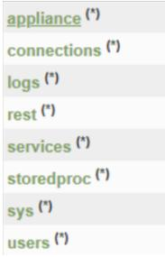
c. Click on the (\*) next to appliance to access the REST command set. The Properties for /appliance dialog is displayed under the initial REST menu. The Output (or command manual help) section describes the commands that the REST API can send to the device, their usage, and their parameters.
