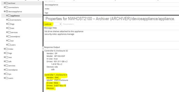
2. Execute the raidNew command with the following parameters using the controller number and the enclosure number you just recorded.
