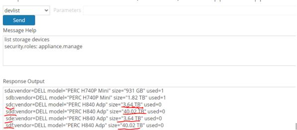
5. SSH to the Network Decoder and use the lsblk command to confirm the block device sizes. The smaller block devices are always allocated to decodersmall and larger devices are allocated to
