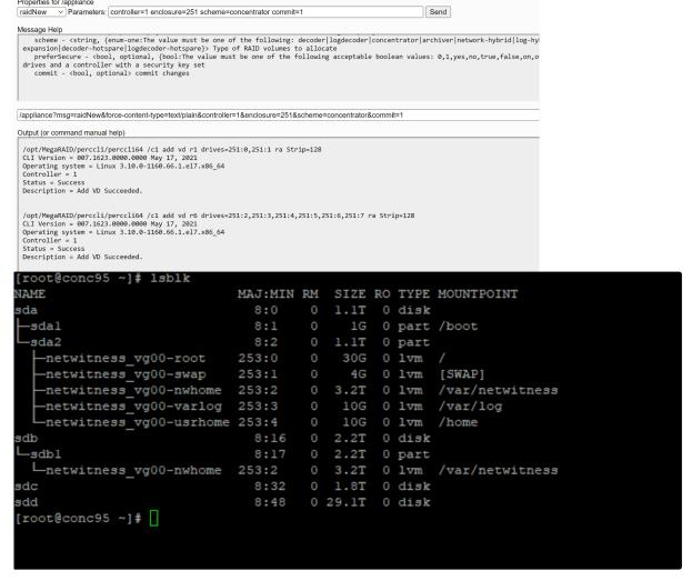
3. Execute the partNew command to create the **concentrator** partition first with the following parameters. You must create the **concentrator** volume before **index** volume or it will fail.
