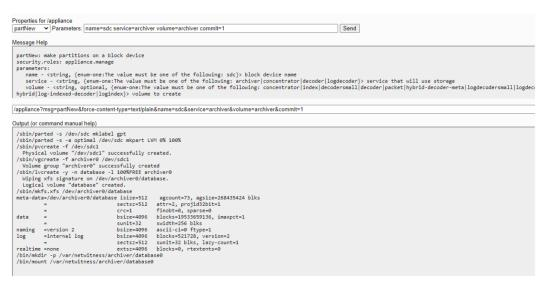
5. Execute the srvAlloc command with the following parameters to allocate the space to the archiver service. This adds storage to the archiver service configuration and restarts the service every time it is executed.
