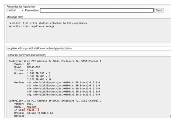
2. Execute the raidNew command with the following parameters using the controller number and the enclosure number you just recorded.
