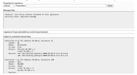
2. Execute the raidNew command with the following parameters using the controller number and the enclosure number you just recorded.
