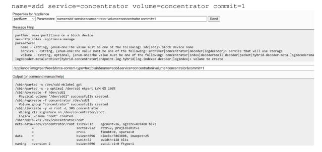
4. Execute the partNew command with the following parameters to create an index on SSDs.
