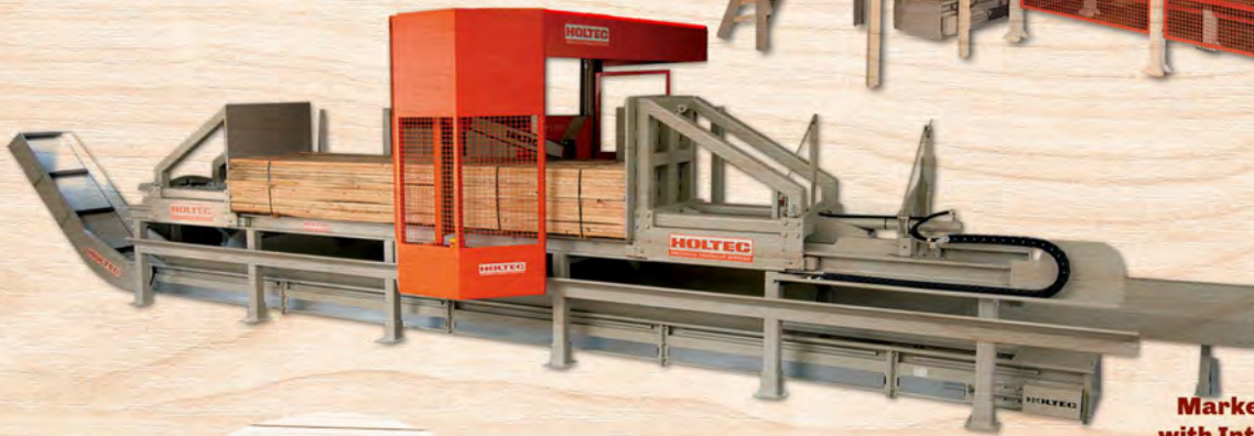
AUTOCUT® High-Volume Automated Crosscutting with programmable PLC Controls
