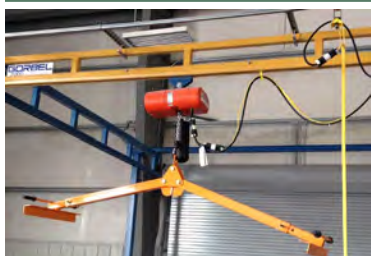
New Wall Panel Lift
