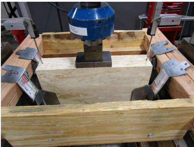
DGT Firewall Hanger Test Failure
