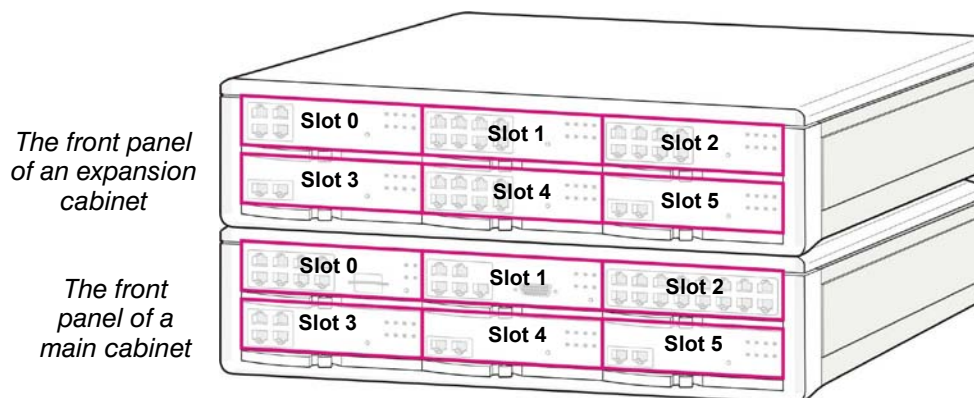
Figure 3.1 Front Panel Configuration
