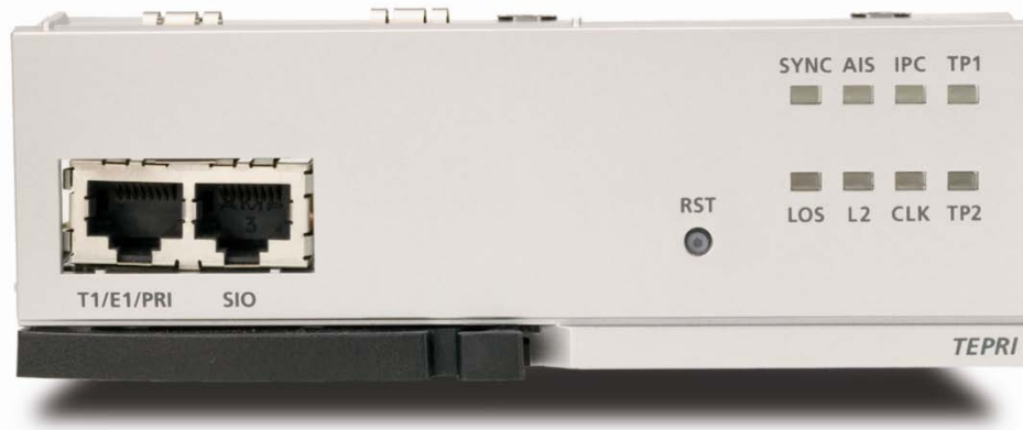
Figure 3.20 Front View of the TEPRI
