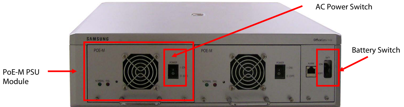
Figure 5.4 Front View of OS 7150 Cabinet
