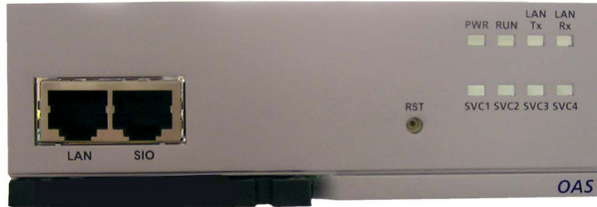
Figure 3.45 Front View of the OAS
