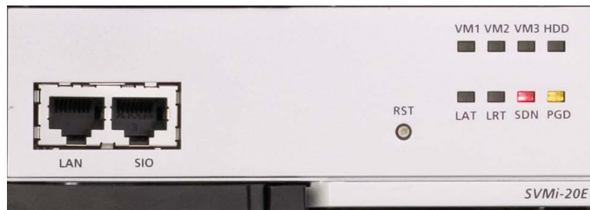
Figure 3.49 SVMi-20E LED Indications
