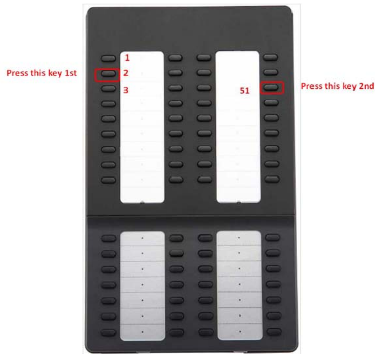
Figure 7.30 Setting-Up SMT-i5264 AOM
