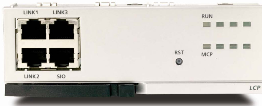
Figure 3.9 Front View of the LCP
