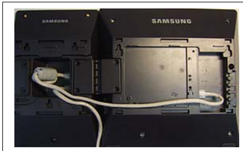
Figure 7.29 Attaching SMT-i5264 AOM to phone
