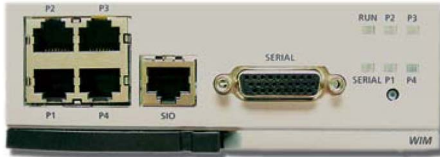
Figure 3.34 Front View of the WIM Board
