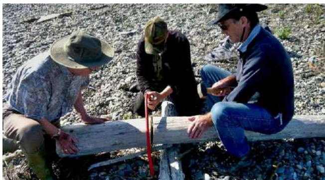
figure 14: Sawing a transverse section through some timber riddled with boreholes. (photo: Jan Light)
