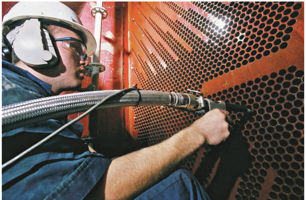
Conco Technician Performing an Eddy Current Test on a Main Steam Condenser
