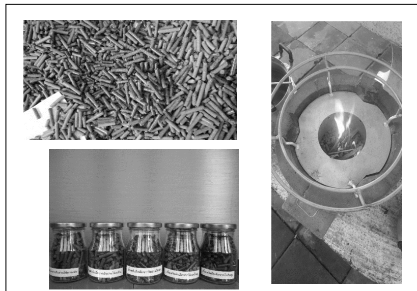
Figure 4 Torrefied Pellet and Boiling test with cooking stove
