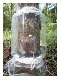
Cylindrical chamber for CH4 flux measurement
