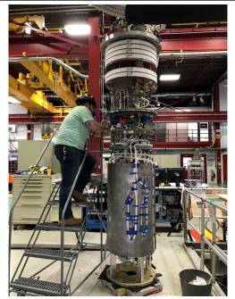
Figure 1. The 60-mm aperture dipole demonstrator MDPCT1 being prepared to cold tests. The magnet reached the record field of 14.5T in June 2020.
