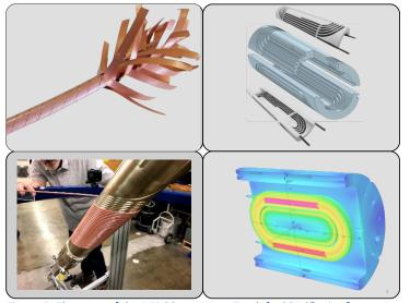
Figure 5. Elements of the REBCO program. Top left: CORC<sup>®</sup> wire from Advanced Conductor Technologies. Top right: Novel "COMB" concept for stress management [13]. Bottom right: first test of REBCO racetrack tapewound coils tested in BNL's 10T common coil magnet. Bottom left: winding of "C2", a CORC-based CCT dipole.
