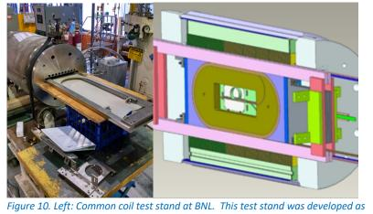
Figure 10. Left: Common coll test stand at BNL. This test stand was developed as part of an SBIR with particle Beam Lasers. Right: An HTS insert coll being placed into the common coll test setup. This hybrid test was also funded as part of an SBIR with Particle Beam Lasers.
