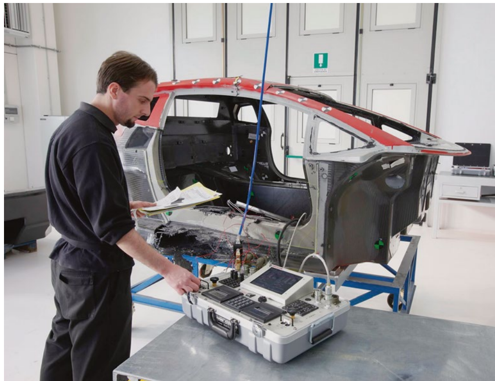
FIGURE 1 Lamborghini deploys their so-called Flying Doctors to repair CFRP structures at the customer's location (© Lamborghini)
