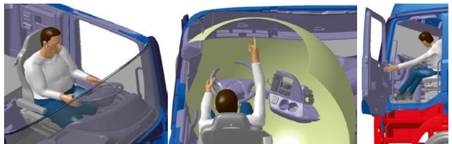
FIGURE 1 Optimising seating design in the commercial vehicle by means of the Ramsis manikin (© Human Solutions)
