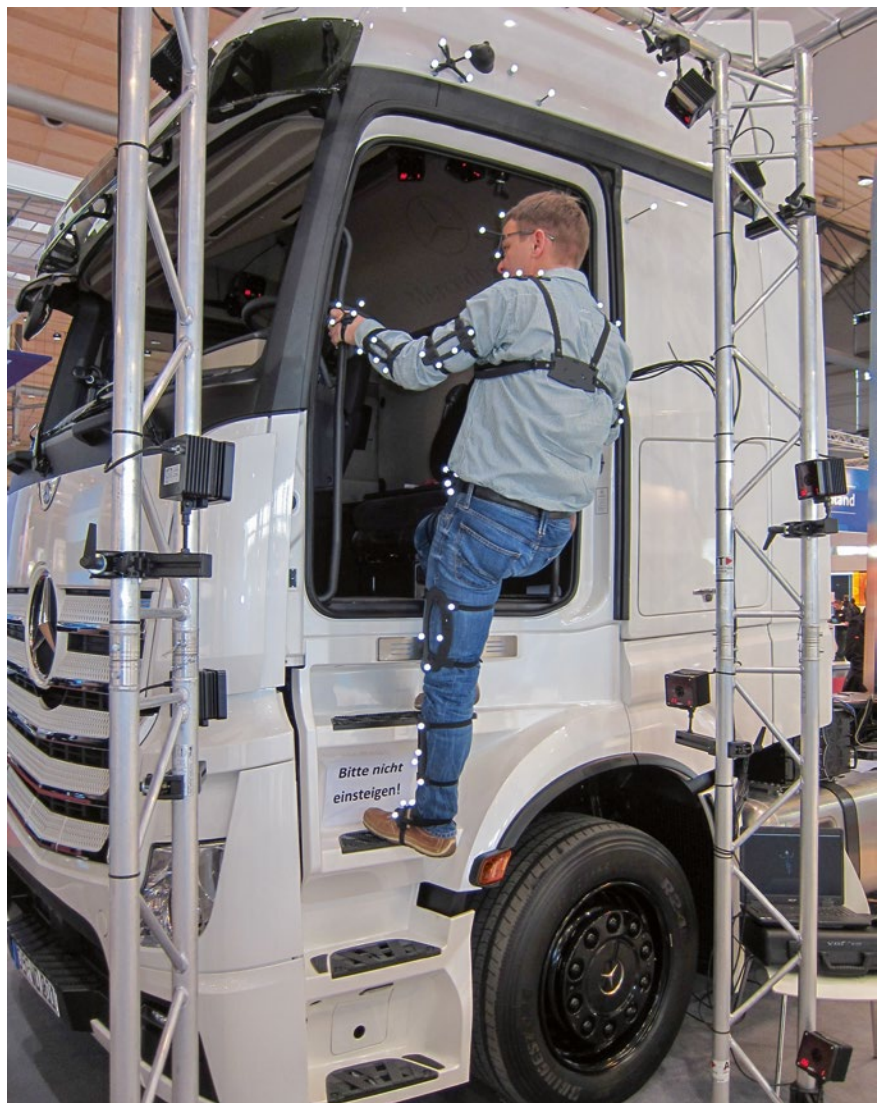
FIGURE 3 Motion capturing at the real vehicle with the optical motion capture system and the reflective markers on the test subject (© Daimler)
