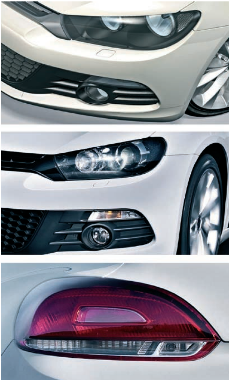
Figure 2: The lighting concept: standard halogen headlights (top), the optional Bi-xenon lights (middle) and the rear lights (bottom)
