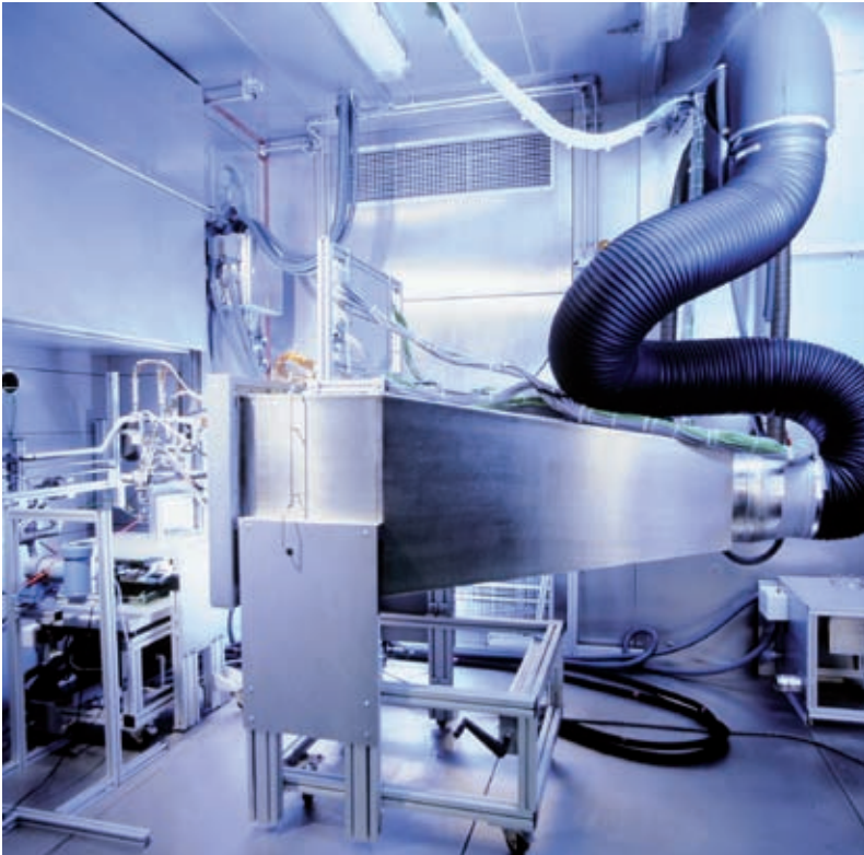
Figure 1: Climatic chamber for simulating the vehicle environment during the measurement of R744 A/C circuits; the climatic chamber is part of the R744 system test facility
