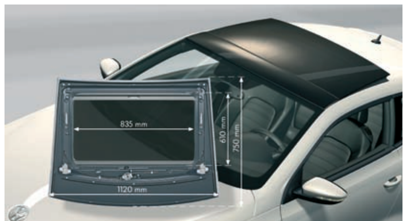
Figure 4: The panoramic vent roof's glass pane is embedded in a plastic frame made from fibre-reinforced PUR
