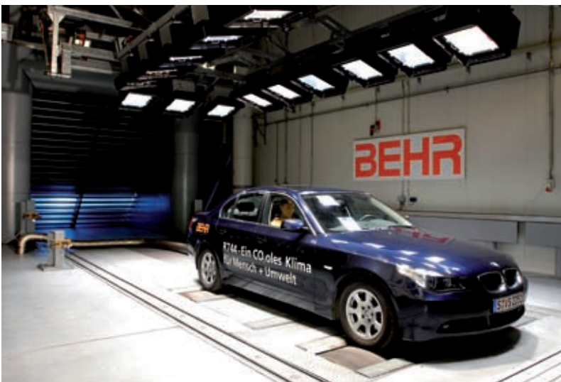
Figure 2: Cooldown measurements in the climatic wind tunnel: with the help of the adjustable solarium, every possible type of solar radiation into the vehicle cabin can be simulated
