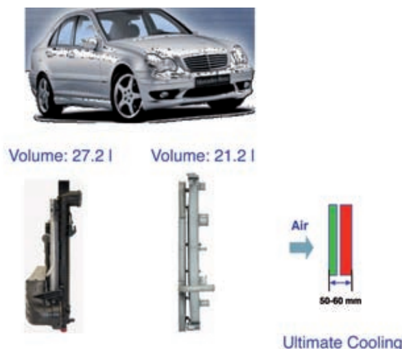
Figure 3: Front-end cooling module of the demo car
