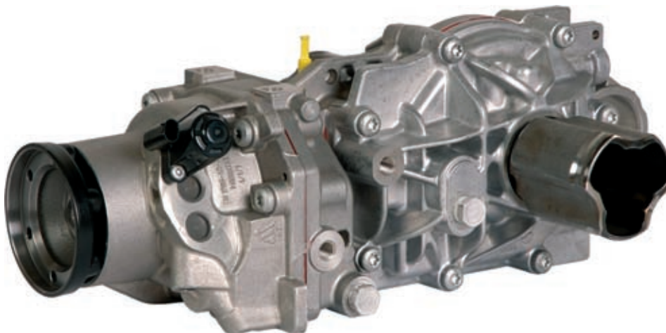
Figure 8: AWD coupling, self-actuating, hydraulic, active control
