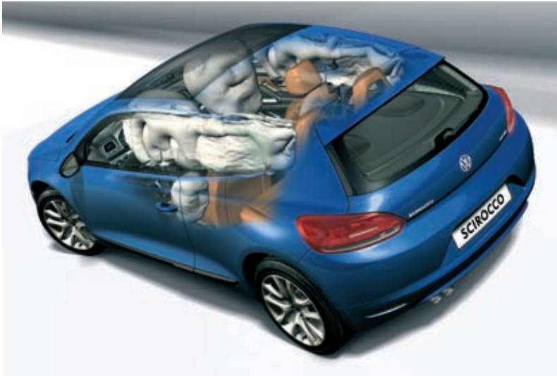
Figure 8: The airbag system includes driver and front passenger airbags, head airbags and side airbags
