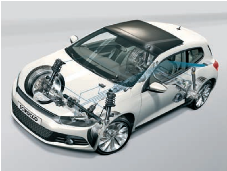
Figure 5: The Scirocco chassis is based on modules from the Volkswagen modular kit
