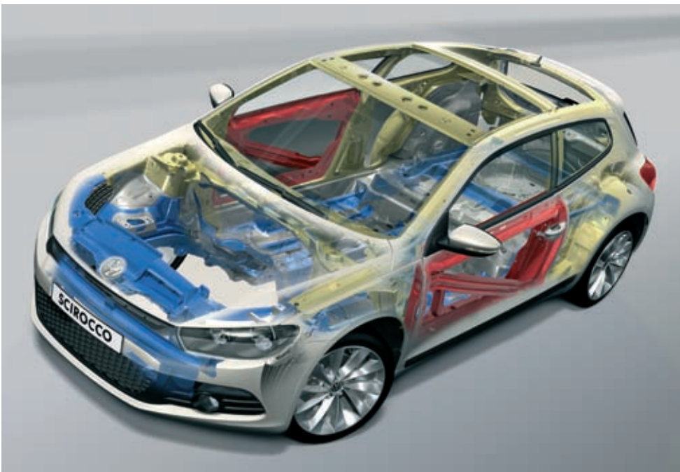
Figure 7: Form-hardened, highest-strength sheet steel increases chassis strength and rigidity
