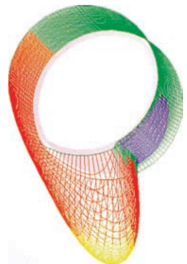
Figure 4: Hydrodynamic pressure distribution of a radial friction type bearing made of bronze (standardized using p_{\max}^* )
