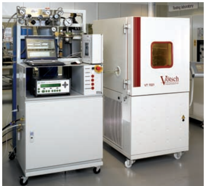
Figure 3: Permeation measurement chamber for CO 2
