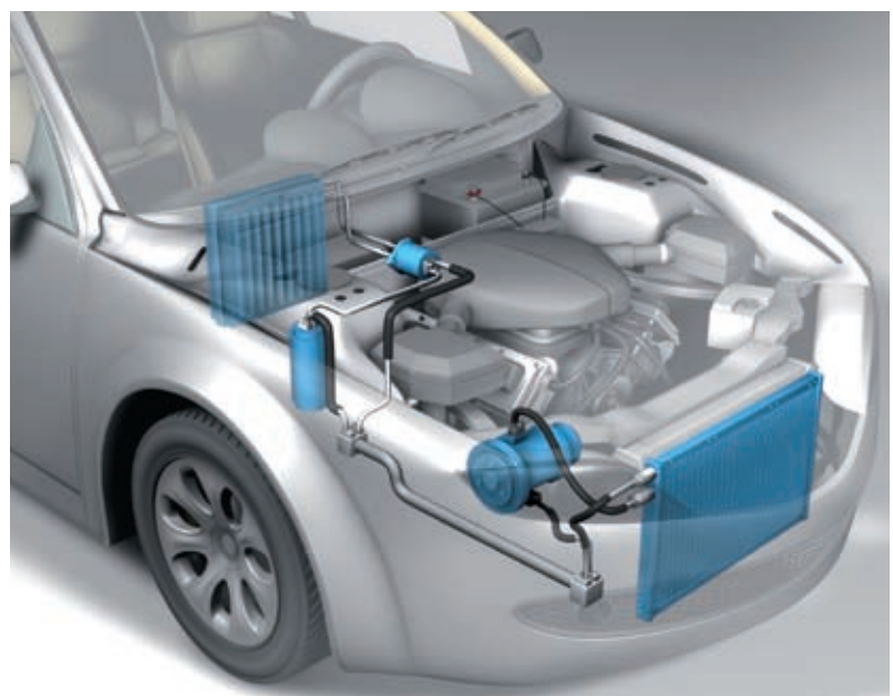
Figure 1: Schematic presentation of a CO 2 air-condition system
