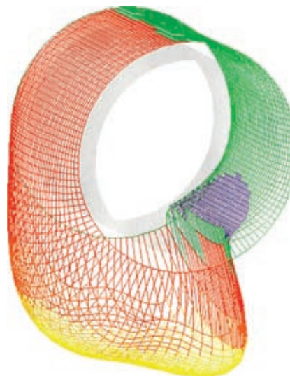
Figure 3: Hydrodynamic pressure distribution of a radial friction type bearing made of a plastic compound (standardized using p_{\max}^* )
