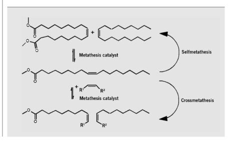
FIGURE 2 Self- and crossmetathesis reactions of oleic acid methyl ester (© Thünen Institute of Agricultural Technology)
