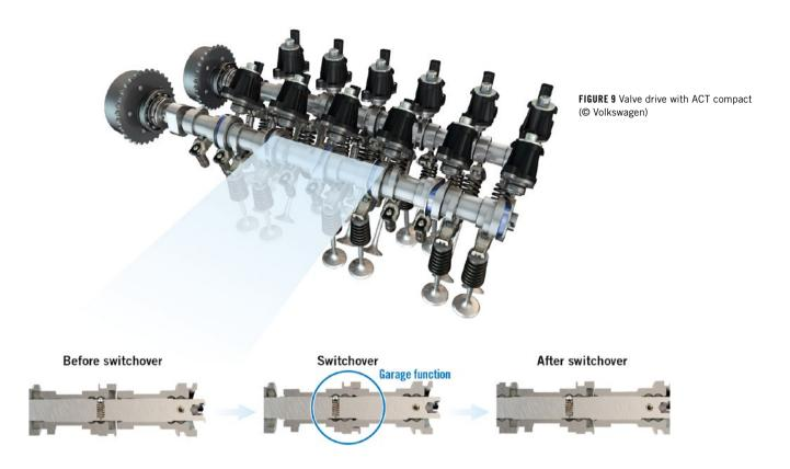
the cylinders are deactivated, a so-called zero-lift cam with a 360° base circle rotates above the rocker arms without actuating them.
