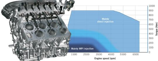
FIGURE 3 Engine mapping for direct and MPI injection when the engine is warm (© Volkswagen)
