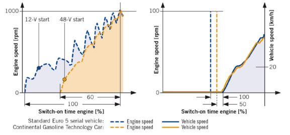
FIGURE 1 Improved engine start and drive-off behaviour of the Gasoline Technology Car compared with the Euro 5 production vehicle (© Continental)
