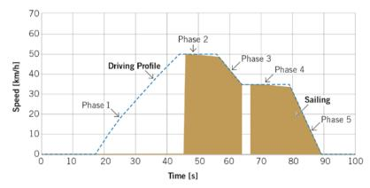
**FIGURE 6** Schematic illustration of a driving profile in connection with sailing periods (© ZF)
