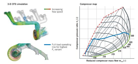
FIGURE 7 Transient 3-D CFD simulation of outlet ports, exhaust manifold and twinscroll turbine (© Volkswagen)
