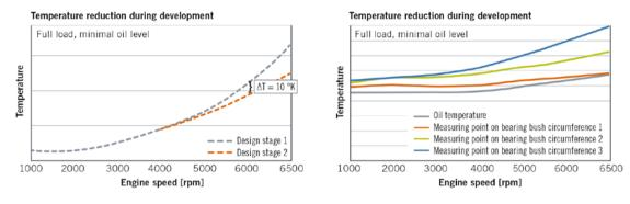
FIGURE 2 Temperature of the bearing bushes, schematical (© Volkswagen)
