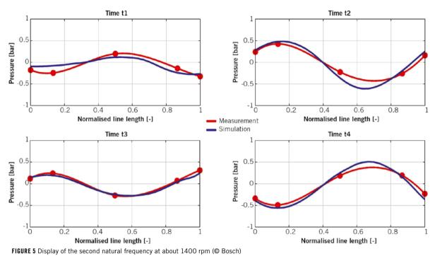
an analytic approach, an observation of the system with a test bench was done. Beyond that, a system simulation with a commercial tool was realised.
