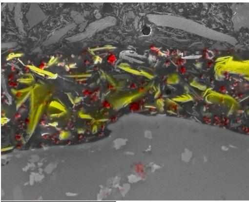
FIGURE 1 Micro section depicting the individual components of the coating EcoTough-New Generation (© Federal-Mogul)
