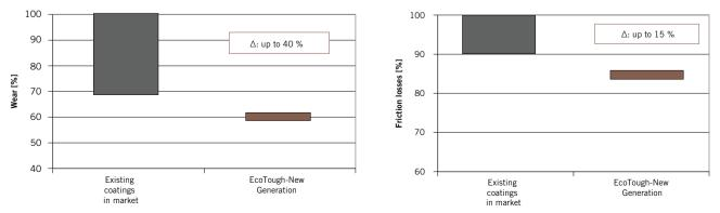
FIGURE 2 Wear and friction of the EcoTough-New Generation skirt coating for gasoline engines as compared to the market standard (© Federal-Mogul)
