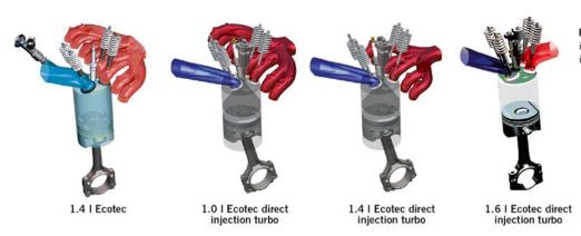
FIGURE 5 Combustion chambers, injection and channels of the individual gasoline engines (© Opel)
