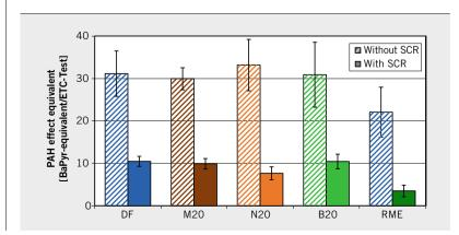
FIGURE 6 Effect equivalent of PAH emissions from particulate and condensate of the OM 904 LA in the ETC test (© Thünen Institute of Agricultural Technology)
