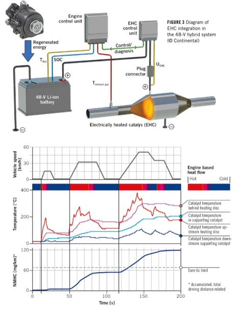
FIGURE 4 NMHC emission behaviour with a consistent engine-off strategy with Emicat compared with a conventional catalyst (© Continental)
