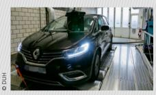
Testing the NO<sub>x</sub> emissions of a Renault Espace 1.6 dCi
