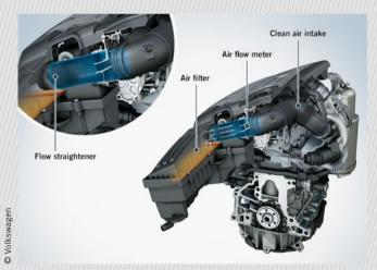
A flow transformer is intended to help clean up the EA 189 diesel engines affected by the emissions scandal
