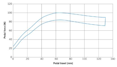
FIGURE 5 Pedal curve of a clutch-by-wire application with a pedal force simulator for a diesel application with a maximum torque of 450 Nm (© ZF)
