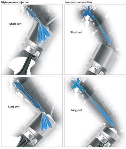
FIGURE 4 High and low-pressure injection spray in short and long port (© Volkswagen)
