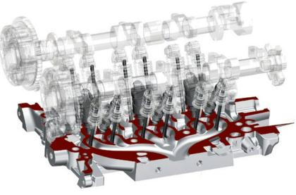
**FIGURE 4** Cylinder head with roller cam follower valve train and integrated exhaust manifold (© Opel)
