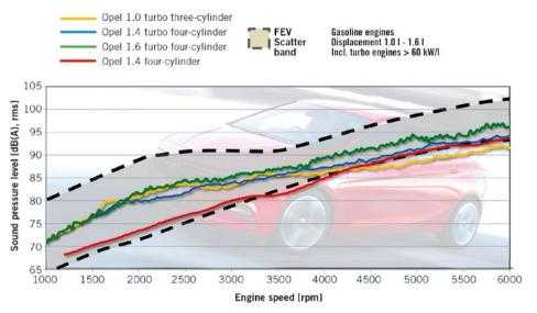
FIGURE 2 Smooth and quiet: the sound pressure level over gasoline engine speeds (© Opel)
