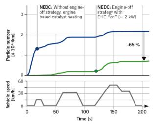
FIGURE 5 Particulate emissions during the first 200 s in the NEDC (© Continental)
