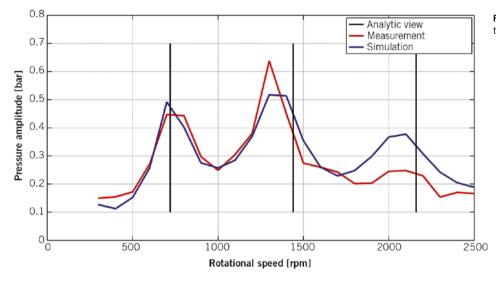
FIGURE 3 Pressure amplitude inside the low pressure line (© Bosch)
