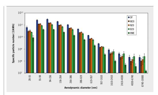
FIGURE 5 Particle size distribution of fossil diesel fuel, 20 % blends of both metathesis fuels and biodiesel in DF, and neat biodiesel, tested in an OM 904 engine with SCR catalyst (ETC test) (© Thünen Institute of Agricultural Technology)
