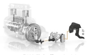
Clutch-by-Wire from ZF means important functions previously reserved for automatic transmission and automated gearboxes are now possible with manual gearboxes for the first time.
