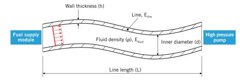
**FIGURE 1** Flexible line between fuel supply module and high pressure pump (© Bosch)
