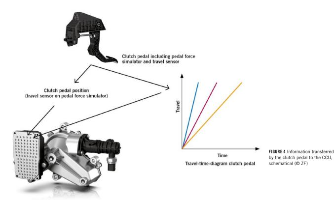
customer acceptance, because drivers operate the shift lever and the clutch pedal in the familiar way. To achieve this, CBW requires a sensor system that measures continuous parameters such as actuation speed and position, **FIGURE 4**.
