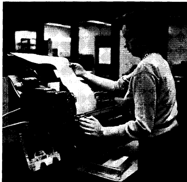
Below, William Cahill removes one of 13 piles of cards just divided by the sorter. Right, Marilyn Brandhagen checks to see that the tabulator is printing correctly.
