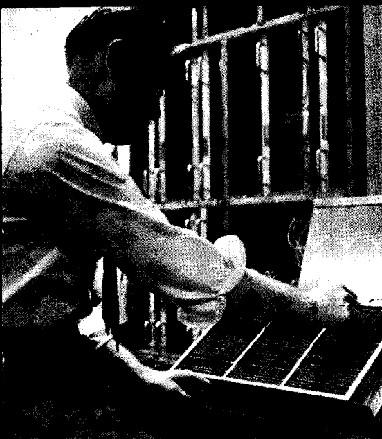
The board Harold Ludke is wiring directs the operations of the tabulator.
