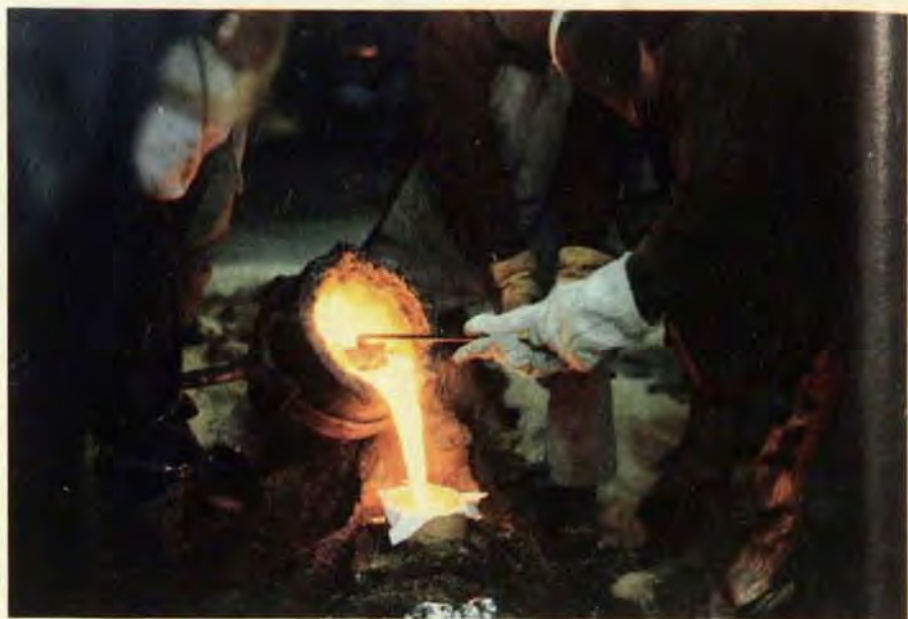
Iron-pour blood is what they say infects Wayne Potratz's students after they attend their first pour, where iron is heated to 2,800 degrees in an open furnace, then poured from ladles to molds. Students have been returning for sixteen years.
