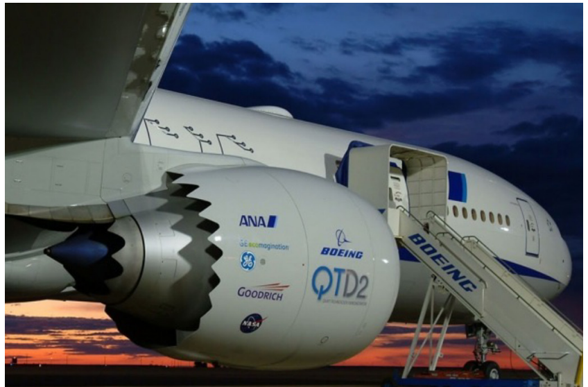
Figure 1: One of several serrated nozzle designs tested by Boeing's Quiet Technology Demonstrator aircraft.
