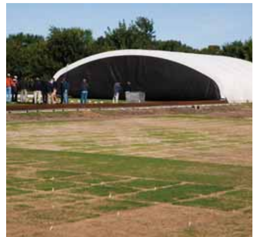
Grass cultivars are tested at the St. Paul campus, where this sliding cover is placed over grass plots whenever it rains. Unprotected plots outside the cover provide comparison. Successful drought-tolerant varieties will save water and lower irrigation costs for golf courses, athletic fields, cemeteries, and lawns.
