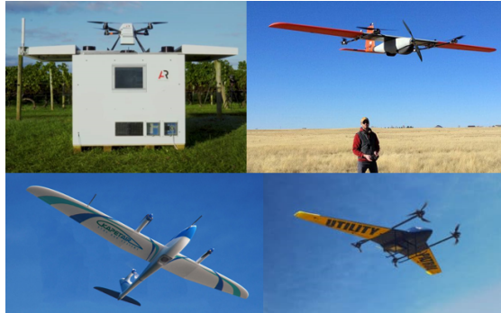
Figure 1.2: Examples of VTOL aircraft include (Top Left) American Robotics’ self-managed UAV system for precision agriculture, (Top Right) Lynx VTOL UAV from Swift Radioplanes, LLC, (Bottom Right) a utility inspection platform from ULC Robotics Inc., and (Bottom Left) the KapetAir VTOL UAV.
