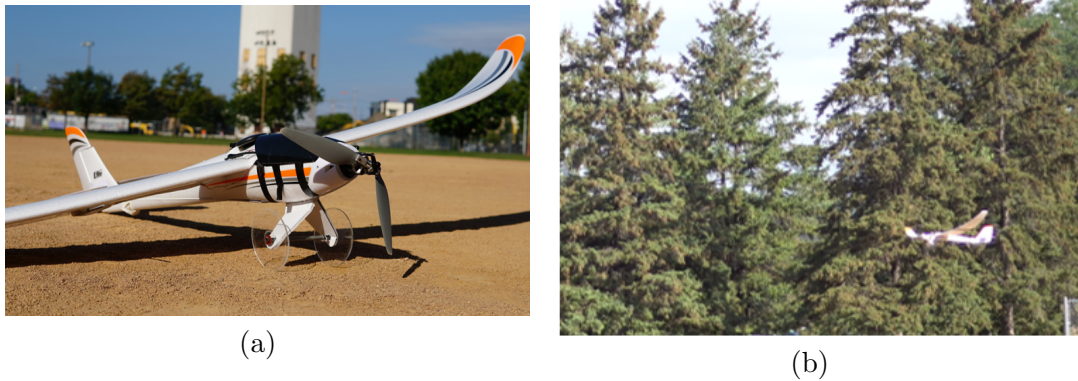
Figure 4.3: (a) The modified E-flite Radian modified with custom hardware for testing VPP performance. (b) The modified E-flite Radian during a takeoff maneuver on one of the flight tests.
