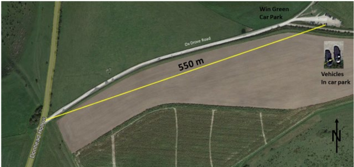
Figure A1: Measured line using the Google earth Ruler Tool. The line is 0.55 km long and bearing of 251.28° from side-mirror of vehicle in the Win Green car park to the intersection of Ox Drove Road and Donhead Hollow Road. Estimated error of the bearing is about \pm 0.16^\circ .
