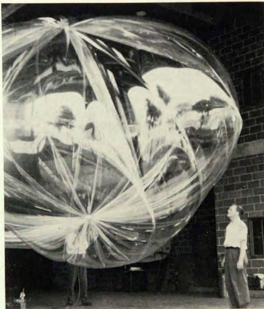
A BALLOON IS filled with air to test its expansion.
