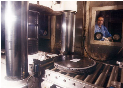
Figure 6.2: Photographs of the interior of the Dounreay Waste Receipt, Assay, Characterisation and Supercompaction (WRACS) facility, showing compaction of LLW drums into thin “pucks” (left), and filling of a HHISO container with compacted LLW drums (right).
