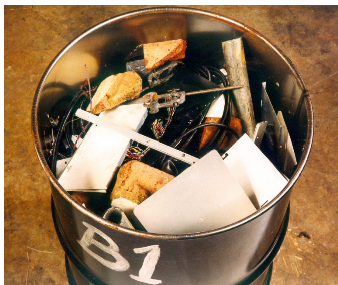
Figure 4.1: Photograph showing typical contents of a drum of Dounreay LLW.
