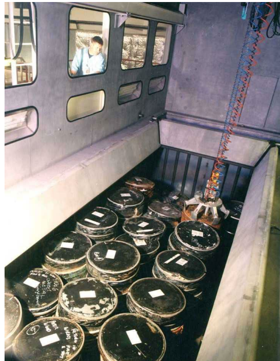
Figure 6.2: Photographs of the interior of the Dounreay Waste Receipt, Assay, Characterisation and Supercompaction (WRACS) facility, showing compaction of LLW drums into thin “pucks” (left), and filling of a HHISO container with compacted LLW drums (right).
