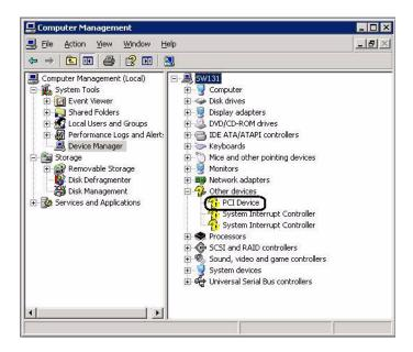
Step 2. Select a PCI Device entry, right-click and select Properties to display the PCI Device Properties window.
