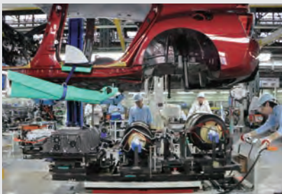
Installing FC stack and tanks
