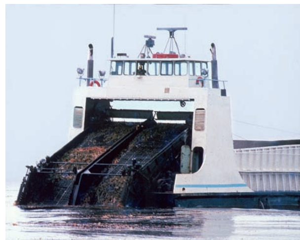
FIGURE 1 Kelp-cutting vessel harvesting giant kelp, Macrocystis , off the Pacific coast of California. Alginates extracted from the harvested kelp are used in many foods and cosmetics. Photograph by Michael S. Foster.
