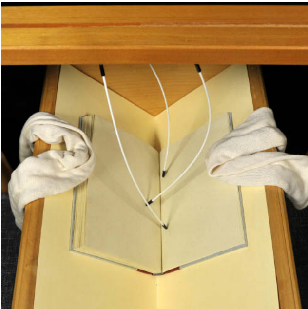
Fig. 4. Three shimbari sticks applying pressure in multiple directions inside a book gutter.
