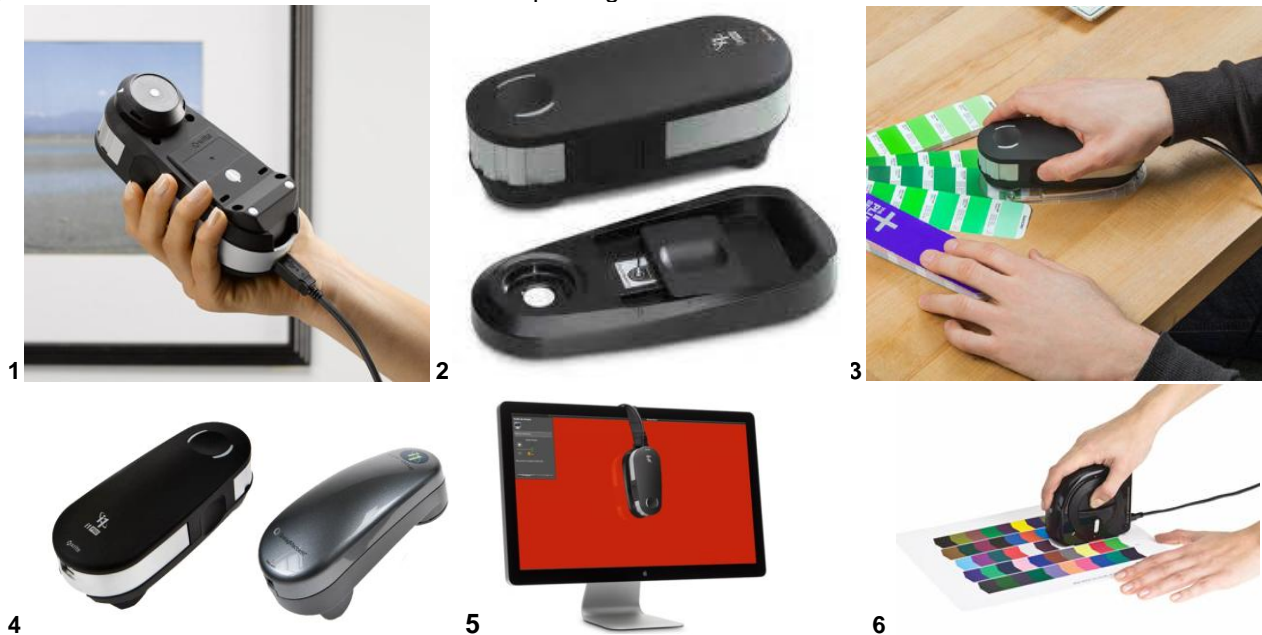
Figure 18 – 1: i1Pro2 with the incident light measurement cap, used for measuring light intensity (Lux) and color temperature (CCT) in degrees Kelvin (°K). 2: i1pro2 off its base showing the calibration tile. 3: i1Pro2 being used to measure paint swatch. 4: Comparison of i1Pro (left) and i1Pro2 (right) not on their bases, which has the calibration tile. 5: i1Pro2 being used to calibrate a monitor. 6: X-Rite ColorMunki ($450) spectrophotometer measuring a color target for printer calibration.
