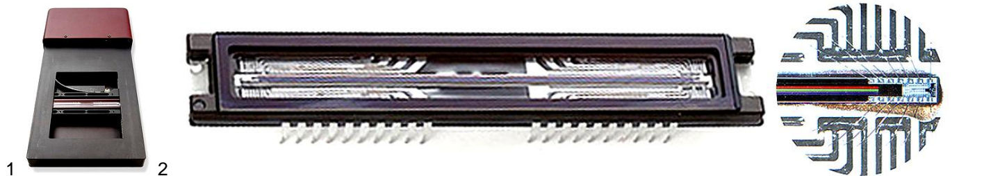
Figure 9 - 1: BetterLight scanback with the sensor parked mid-scan. 2: enlargement of the trilinear CCD array with individual R, G & B rows of pixels. Far Right: end of the array enlarged to show the actual red, green and blue bands of pixels all from BetterLight website.
