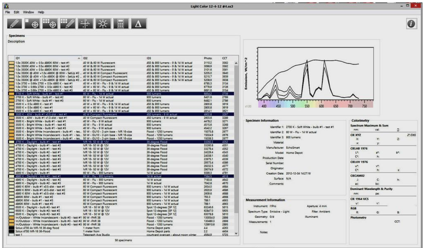
Figure 19 – In SpectraShop v4.0.1, working with a collection of light bulb spectra currently use in my Conservation Studio, for color matching while inpainting artworks or of matching an original artifact to its digital facsimile. Note the 4 spectra open in the spectral viewer (i) the top smooth hump is a MR-16 quartz-iodine bulb with a diachronic reflector and (sometimes) a filter on the sealed front, this particular bulb is labeled 4700°K delivering 4352°K at roughly 33,000 Lux intensity 12" from the bulb; (ii-vi) are modern compact fluorescent (CF) bulbs from Home Depot labeled (top) 60W-Daylight, delivering 4618°K CCT at 7384 Lux with many characteristic phosphor spikes in the spiky spectra, (middle) 40W-3500°K and delivering 3239°K CCT at 4903 Lux with the same spiky spectra and (bottom) 60W-Soft White delivering 2739°K CCT at 6854 Lux with the same spiky spectra. Spiky spectra often yield poor Color Rendering Index (CRI) values, while smooth spectra with a color temperature near 5000°K have high CRI.
