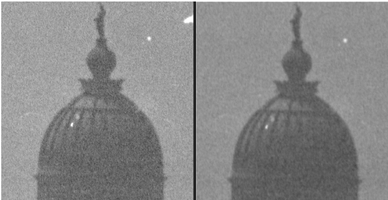
Figure 24: Scanned by author using both dry (left) and wet mount (right) techniques, at 4800 ppi optical resolution, using 16-bit B&W dynamic range, on an Epson 4870 flatbed. Film grain should look soft because it is perceived through the thickness of the emulsion layer and is soft in reality. Note how the wet-scanned image actually has better definition between the dark rib and the gray panel on the far left of the dome. Also note how the dry scanned grain detracts from resolving information in the 100 year old film; the image is much noisier. Some believe that the dry scanned image looks sharper because the film grain appears sharp, but comparing the images will show more image information in the wet scanned image.
