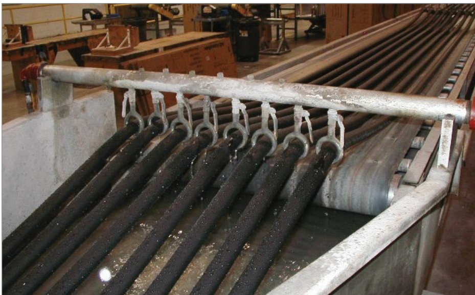
Foam insulation emerging from direct cooling water bath
