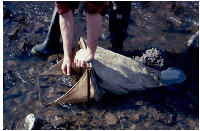
Figure 41. Surber sampler, showing the investigator removing a rock from the sampling area. The opening of the net faces upstream and the net catches organisms dislodged during sampling. Photo by Ray Drenner, with permission.
