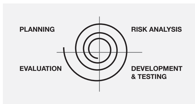
Figure 1.4: Spiral model methodology (Boehm, 1988)
