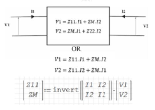
Figure 17-9 Mutual Inductance Calculated With Semi-Analytical Approach
