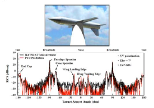
Figure 11-51: Measured and Calculated RCS of Johnson Generic Aircraft Model
