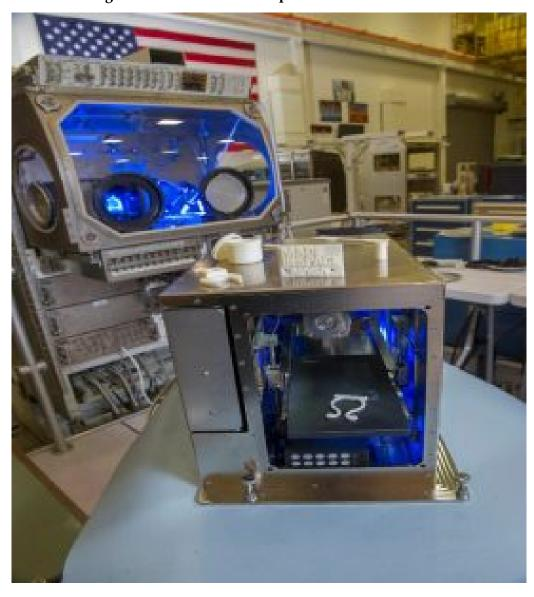
Figure 15-5: International Space Station's FDM Printer
