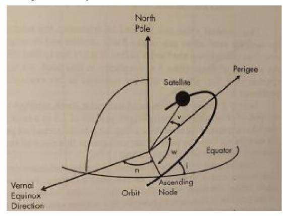
Figure 10-1 The Ephemeris defines the satellite's location with six factors.
