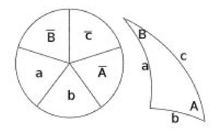
Figure A-3: Napier's Rules for Right Spherical Triangles
