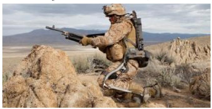
Figure 5-15 The Human Universal Load Carrier, or HULC
