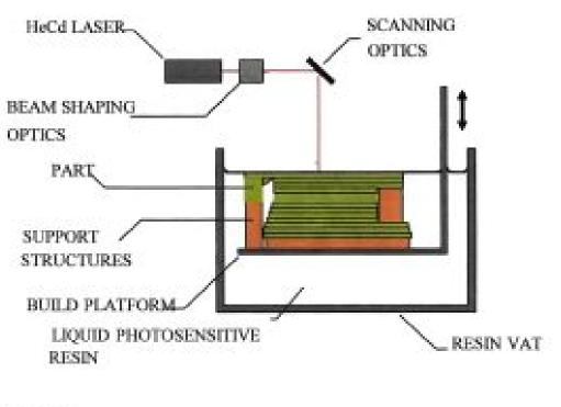
Figure 15-11: Schematic of the Stereolithography Process
