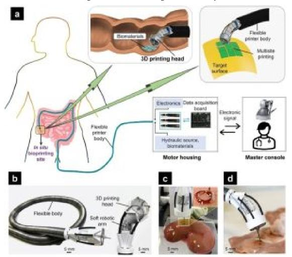
Figure 1-17: 3D Printing inside the body
