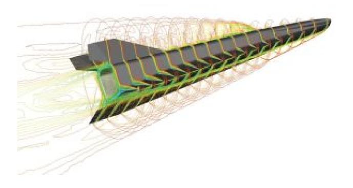
*Note:* "Passing the speed of sound compresses air flowing over an airfoil, creating a shockwave.- the "sonic boom" Waveriders use the shockwave to increase their lift, essentially surfing on a wave of pressurized air." "(U.S. Naval Institute, 2020)
