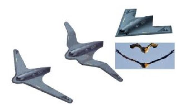
*Note:* Different morphing configurations can provide the ultimate configuration relative to the action performed. The above image has standard flight, Lottering, and dash configurations.
