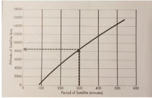
Figure 10-2 Altitude of a Circular Satellite is a Function of its Orbital Period
