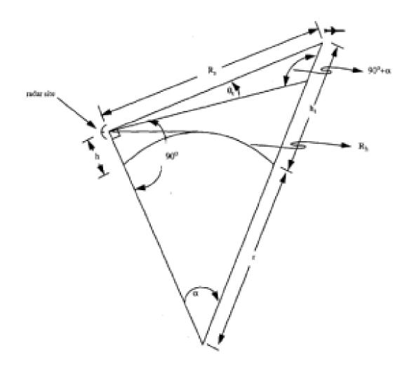
Figure 11. Start range and elevation angle from radar to aircraft
