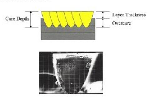
Figure 15-10: Layer-to-layer Bonding and a Scanning Electron Micrograph Showing the Cross Section of a Cured Line
