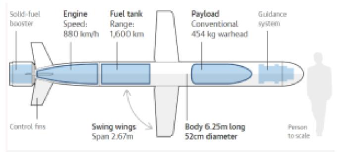
Guardian graphic | Source: US Navy | Conversions: Speed 550 mph, Range 1,000 miles, Warhead 1,000 lb, Span Bft 9in, Body 20ft 6in by 20.4in
