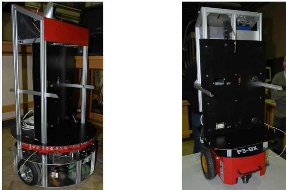
Figure 5-7: Nubot platform with 4 drawers (left) and Pioneer Robot platform with 2 drawers in the front side (right)
