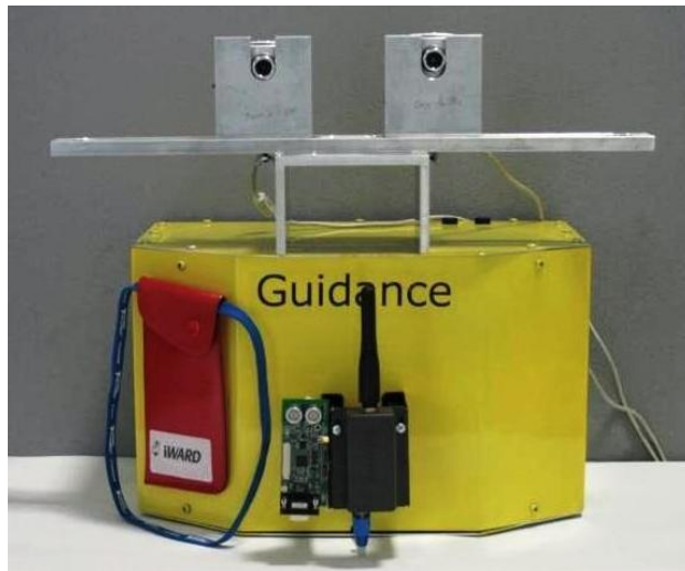
Figure 5-13: Final PGM Hardware Assembly (Exterior).
