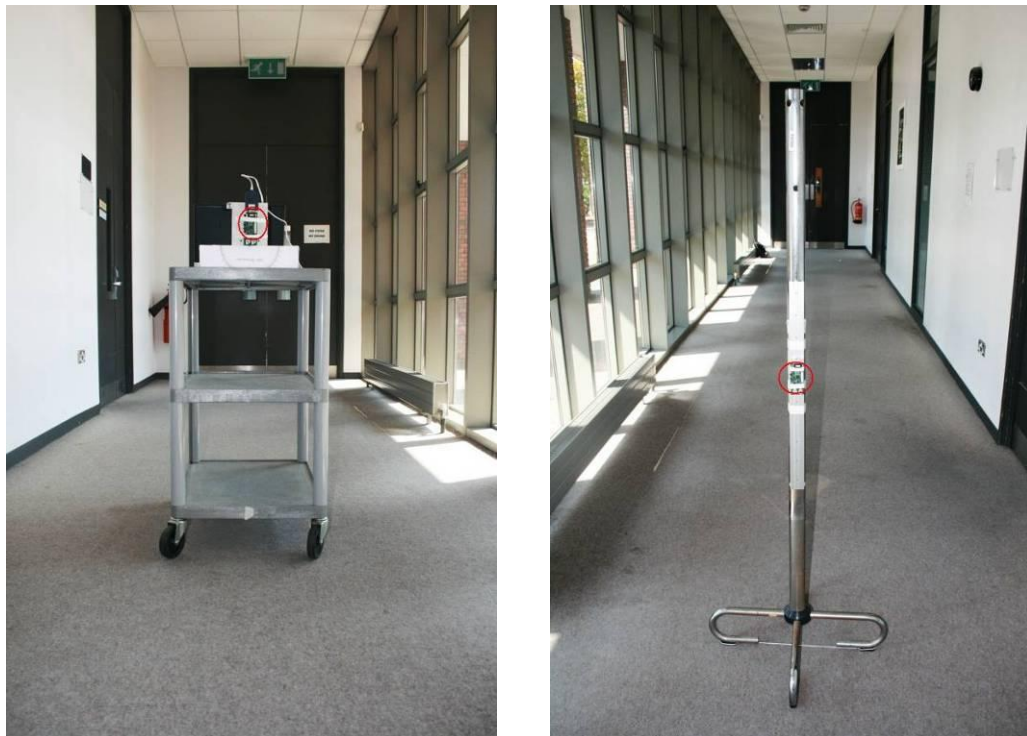
Figure 4-10: Experiment set up in the corridor. The listener is placed on a cart (left) and the beacon is attached to a stand (right).
