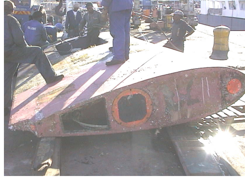
Figure 7.5 Transducer arrangement of the drop keel of R/V “Dr. Fridtjof Nansen”, during 1999, showing orientation of the transducers on the keel.
