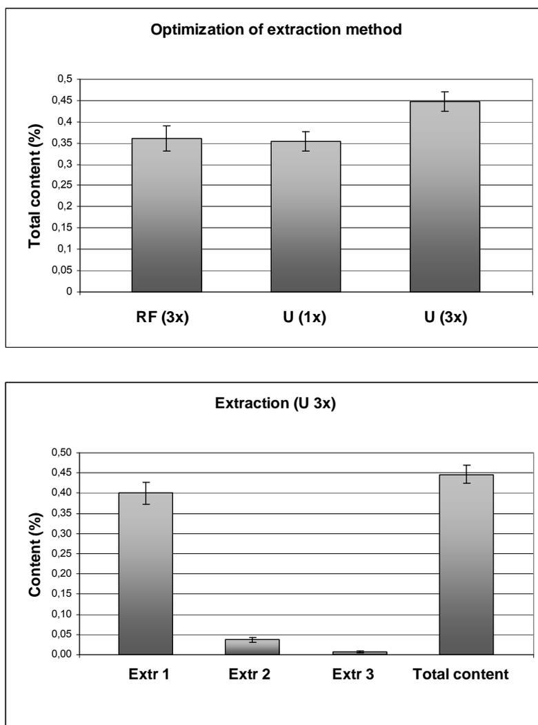
Legend: The upper panel compares the total content of flavonoids after extraction with a mixture of MeOH/water (40/60, v/v) under reflux (RF 3x, 30 min each), extraction for one time by ultrasound (U 1x, 10 min), and extraction for three times by ultrasound (U 3x). For each of the extraction modes three individual samples were tested. The lower panel compares the three extraction steps (Extr 1, Extr 2, Extr 3) by ultrasound (U 3x).
