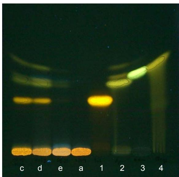
**Fig. 12** TLC analysis of the OWE (chapter 2.2.1, p. 19) of samples **a**, **c**, **d**, and **e** in comparison to the reference substances luteolin (1), apigenin (2), kaempferol (3), and chrysoeriol (4) applying system 2 (chapter 2.3.1 p. 24, table 3) detected with natural product reagent/PEG 400, UV 366 nm
