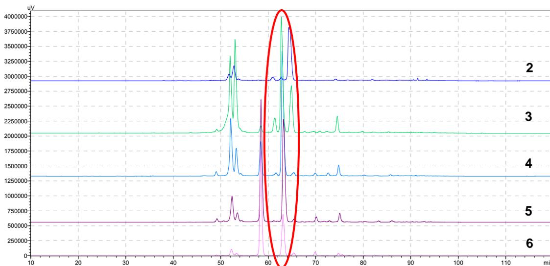
**Fig. 22** HPLC analysis of fractions 2-6 (Fig. 7, chapter 2.2.4, p. 23) on Aquasil<sup>®</sup> C 18 applying the following linear gradient: 0→10% B within 20 min, 10→20% within 60 min, 20→40% B within 20 min, 40→95% B within 10 min at a flow rate of 1 mL/min and a column oven temperature of 25°C; detected at 340 nm
