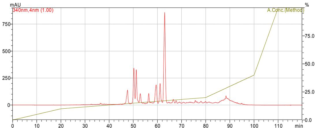
**Fig. 18** HPLC analysis of the OWE (chapter 2.2.1, p. 19) on Aquasil® C 18 applying the following linear gradient: 0→10% B within 20 min, 10→20% within 60 min, 20→40% B within 20 min, 40→95% B within 10 min at a flow rate of 1 mL/min and a column oven temperature of 25°C; detected at 340 nm
