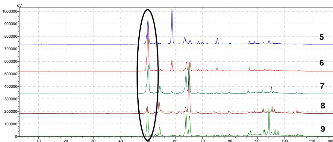
**Fig. 23** HPLC analysis of fractions 5-9 (Fig. 7, p. 23) on Aquasil<sup>®</sup> C 18 applying the following linear gradient: 0→10% B within 20 min, 10→20% within 60 min, 20→40% B within 20 min, 40→95% B within 10 min at a flow rate of 1 mL/min and a column oven temperature of 25°C; detected at 340 nm
