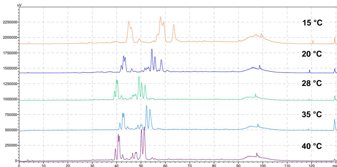
**Fig. 16** HPLC analysis of the OWE (sample **a**, chapter 2.2.1, p. 19) on Phenomenex® Luna Phenyl-hexyl applying the following linear gradient: 0→10% B within 20 min, 10→12% within 5 min, 12→20% B within 60 min, 20→100% B within 10 min at a flow rate of 0.2 mL/min and various column oven temperatures; detected at 340nm
