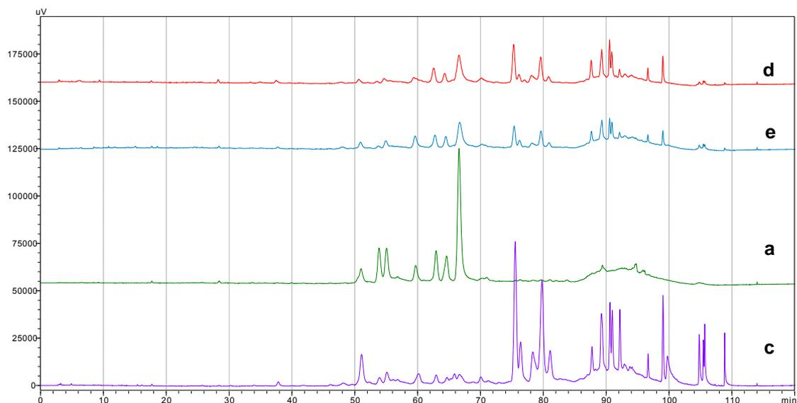
**Fig. 26** HPLC analysis of the OWEs (chapter 2.2.1, p. 19) of samples **a**, **c**, **d**, and **e** on Aquasil® C 18 (5µm particles) applying the following linear gradient: 0→10% B within 20 min, 10→20% within 60 min, 20→40% B within 20 min, 40→95% B within 10 min at a flow rate of 1 mL/min and column oven temperature of 15°C; detected at 340 nm
