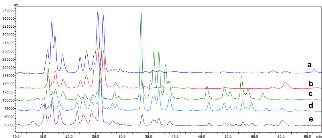
**Fig. 27** HPLC analysis of the OWEs (chapter 2.2.1, p. 19) of samples **a-e** on Aquasil® C 18 (5µm particles) applying the following linear gradient: 15→23.75% B within 58 min, 23.75→29% within 15 min at a flow rate of 1 mL/min and a column oven temperature of 15°C; detected at 340 nm
