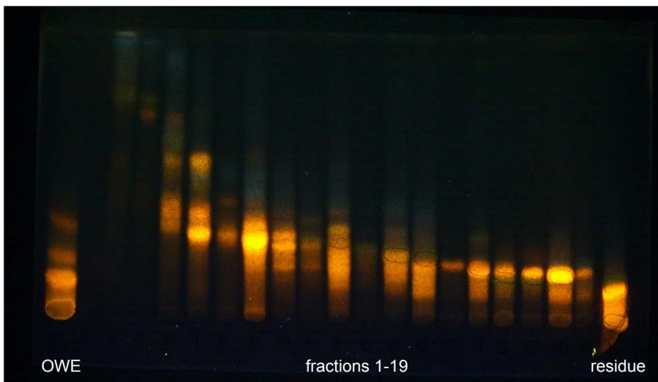
**Fig. 10** TLC analysis of the OWE (chapter 2.2.1, p. 19), the unified fractions 1-19 and the residue obtained by CPC (chapter 2.2.3, p. 20 and publication 2 [22] chapter 3.1. pp. 30-85) applying system 1 (chapter 2.3.1, p. 24 table 3) detected with natural product reagent/PEG 400, UV 366 nm
