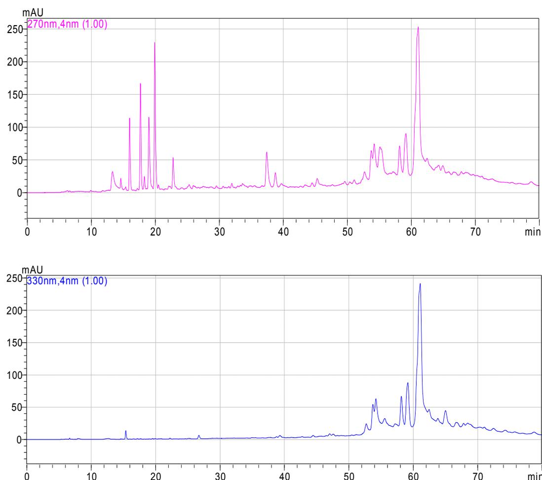
**Fig. 17** HPLC analysis of the OWE (sample **a**, chapter 2.2.1, p. 19) on Aquasil® C 18 applying the following linear gradient: 0→10% B within 20 min, 10→23% within 40 min, 23 isocratic for 15 min, 23→40% B within 10 min, 40→100% B within 5 min at a flow rate of 1 mL/min and a column oven temperature of 25°C; detected at 270 nm (upper panel) and 330 nm (lower panel)
