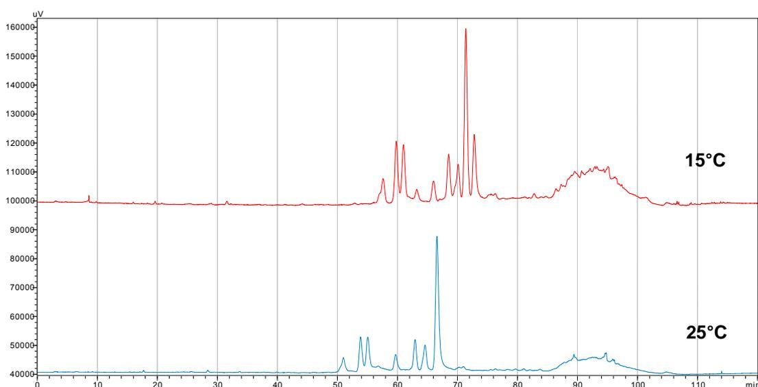
**Fig. 24** HPLC analysis of the OWE (chapter 2.2.1, p. 19) on Aquasil<sup>®</sup> C 18 applying the following linear gradient: 0→10% B within 20 min, 10→20% within 60 min, 20→40% B within 20 min, 40→95% B within 10 min at a flow rate of 1 mL/min and column oven temperature of 15 and 25°C; detected at 340 nm
