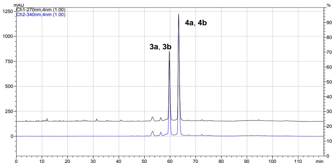
**Fig. 21** HPLC analysis of fraction I (35-42) (Fig. 7, chapter 2.2.4, p. 23) on Aquasil<sup>®</sup> C 18 applying the following linear gradient: 0→10% B within 20 min, 10→20% within 60 min, 20→40% B within 20 min, 40→95% B within 10 min at a flow rate of 1 mL/min and a column oven temperature of 25°C; detected at 270 and 340 nm;
