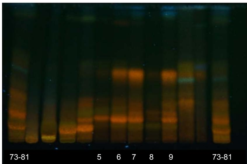
**Fig. 11** TLC analysis of the unified fraction 73-81 obtained by CC of the OWE (chapter 2.2.1, p. 19) on polyamide (chapter 2.2.4, p. 21 and publication 2 [22] chapter 3.1. p. 30-85) and further fractions thereof obtained by CC on Sephadex LH 20 (chapter 2.2.4, p. 21 and publication 2 [22] chapter 3.1. p. 30-85, Fig. 6, p. 21 and Fig. 7, p. 23) applying system 1 (chapter 2.3.1 p. 24, table 3) detected with natural product reagent/PEG 400, UV 366 nm
