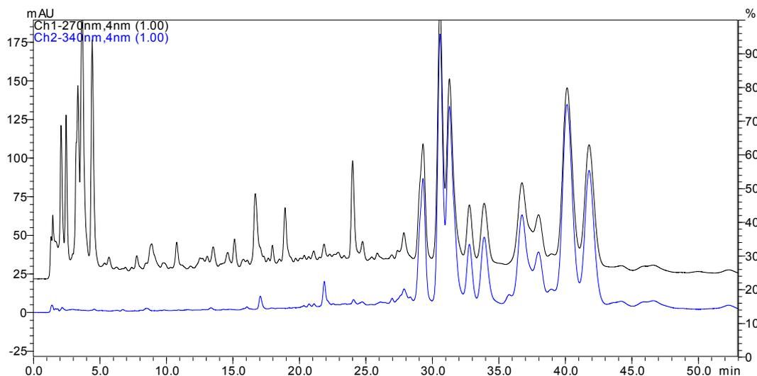
**Fig. 25** HPLC analysis of the OWE (chapter 2.2.1, p. 19) on Aquasil® C 18 (3 $\mu$ m particles) applying the following linear gradient: 2 $\rightarrow$ 14% B within 23 min followed by an isocratic period of 23 min at a flow rate of 0.35 mL/min and column oven temperature of 15°C; detected at 270 and 340 nm
