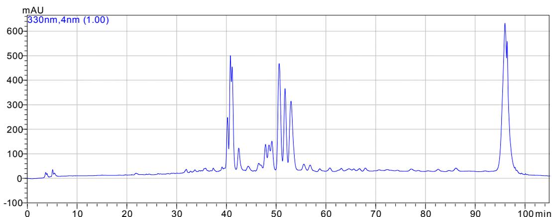
**Fig. 15** HPLC analysis of the OWE (sample **a**, chapter 2.2.1, p. 19) on Phenomenex® Luna Phenyl-hexyl applying the following linear gradient: 0→10% B within 20 min, 10→12% within 5 min, 12→20% B within 60 min, 20→100% B within 10 min at a flow rate of 0.2 mL/min and a column oven temperature of 25°C; detected at 330nm
