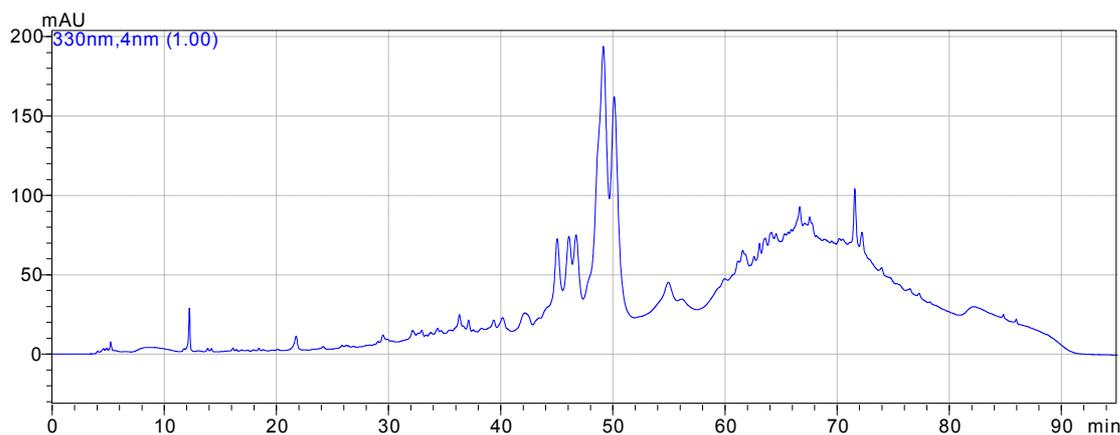
**Fig. 14** HPLC analysis of the OWE (sample **a**, chapter 2.2.1, p. 19) on LiChrospher® 100 RP-18e applying the following linear gradient: 0→15 % B within 30 min, 15% isocratic for 20 min, 15→40% B within 25 min, 40→100% B within 10 min at a flow rate of 1mL/min and a column oven temperature of 25°C; detected at 330nm
