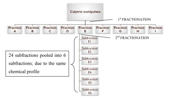
Figure 20. Fractionation scheme for the isolation of compounds from *Calytrix exstipulata* leaf oil.
