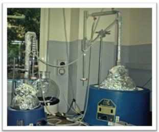
Figure 7. Water steam distillation apparatus.
