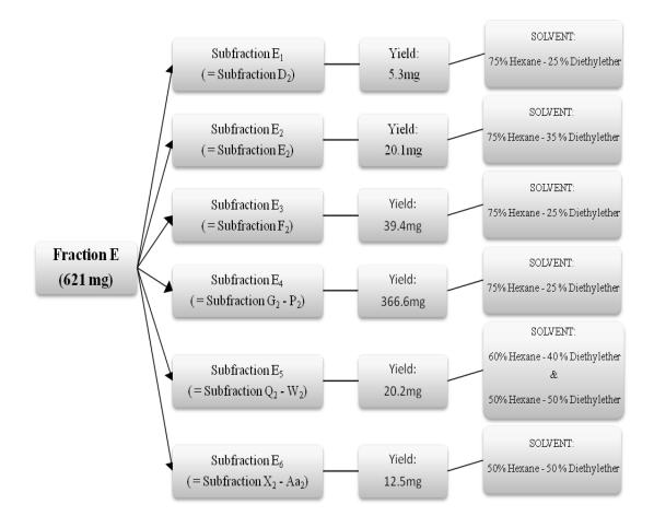
Figure 31. Fractionation scheme for the fractionation of Fraction E.
